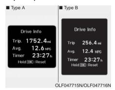
The trip computer mode displays information related to vehicle driving parameters including range, fuel economy, trip meter information and vehicle speed.
