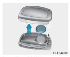
Battery Type: CR2032 To replace the battery:
