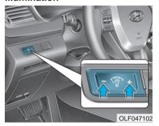
The brightness of the instrument cluster illumination can be adjusted by pressing the illumination control buttons ("+" or "-"), when the Engine Start/Stop button is ON, or when the parking lights are turned ON.
