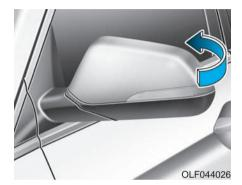
To fold either the left or right hand side view mirror, grasp the housing of the mirror and then fold it toward the rear of the vehicle.
