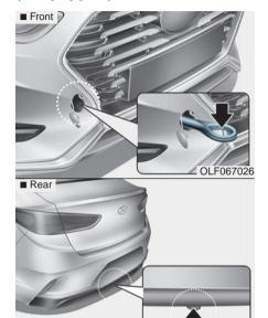
If towing is necessary, we recommend you to have it done by an authorized HYUNDAI dealer or a commercial tow truck service. If towing service is not available in an emergency, your vehicle may be temporarily towed using a cable or chain secured to the emergency towing hook at the rear of the vehicle.
