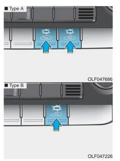
This is used to select the outside (fresh) air position or recirculated air position.
