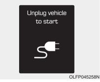
The message is displayed when you start the engine without unplugging the charging cable. Unplug the charging cable, and then start the vehicle.
