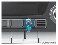
If you push the ECON button while the air conditioning system is working, the air conditioning system will work less and may improve fuel efficiency.
