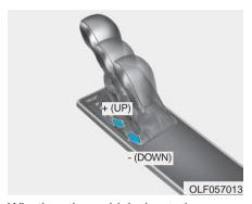
Whether the vehicle is stationary or in motion, manual shift mode is selected by pushing the shift lever from the D (Drive) position into the manual gate. To return to D (Drive) range operation, push the shift lever back into the main gate.
