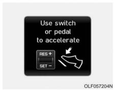
In traffic, your vehicle will stop if the vehicle ahead of you stops. Also, if the vehicle ahead of you starts moving, your vehicle will start as well. However, if the vehicle stops for more than 3 seconds, you must depress the accelerator pedal or push up the toggle switch (RES+ or SET-) to start driving.
