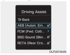
The driver can activate the AEB by placing the ignition switch to the ON position and by selecting 'User Settings', 'Driving Assist', and 'AEB (Automatic Braking System)'. The AEB deactivates, when the driver cancels the system setting.
