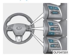
The LCD display modes can be changed by pressing the control switches on the steering wheel.
