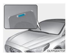
When scheduled charging is set and the normal charger or the portable charging cable (ICCB: In-Cable Control Box) is connected for charging, the indicator lamp blinks (for 3 minutes) to indicate that scheduled charging is set.  When scheduled charging is set, charging is not initiated immediately when the normal charger or portable charging cable (ICCB: In-Cable Control Box) is connected. When immediate charging is required, use the AVN to deactivate the scheduled charge setting.
