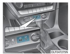
You can use an AUX port to connect audio devices and an USB port to plug in an USB and also in an iPod® port.
