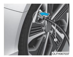
4. Unscrew the valve cap from the valve of the defective wheel and screw the filling hose (3) of the sealant bottle onto the valve.
