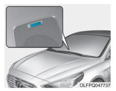
You can monitor the charging status outside of the vehicle when charging the high-voltage battery.
