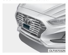
The Smart Cruise Control uses a radar to detect distance to the vehicle ahead.
