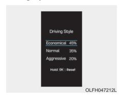
The driving style is displayed when you select "ECO" mode by pressing the DRIVE MODE button.
