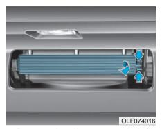
3. Remove the climate control air filter case by pulling out the right side of the cover.
