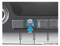
If you press the DRIVER ONLY button( ) and the indicator light illuminates, cold air mostly blows in the direction of the driver's seat. However, some of the cold air may come out of other seats' ducts to keep indoor air pleasant.
