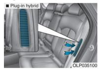
Do not put objects on the left side of rear seat. This could block the battery cooling duct causing battery degradation.
