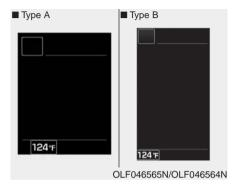
This gauge indicates the current outside air temperatures by 1°F (1°C).
