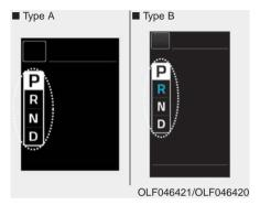
Shift indicator Pop-up (if equipped) The pop-up displays the current shift indicator selected for 2 seconds (P/R/N/D).
