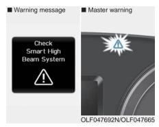
When the Smart High Beam Assist System is not working properly, the warning message will come on for a few second. After the message disappears, the master warning light will illuminate. Take your vehicle to an authorized HYUNDAI dealer and have the system checked.
