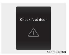
The message is displayed when the vehicle is driven with the fuel filler door opened. Close the fuel filler door and then start driving.
