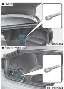
1. Open the trunk, and take the towing hooks out from the tool case.
