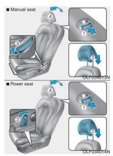
To reinstall the head restraint:
