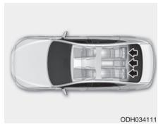
The rear seats are equipped with head restraints all seating positions for passenger safety and comfort.
