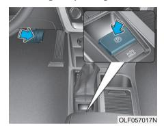
To release the EPB With the Engine Start/Stop button in the ON position.
