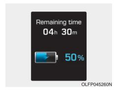
The message is displayed to notify the remaining time to fully charge the battery.
