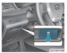
(ESC) system helps to stabilize the vehicle during cornering maneuvers. ESC checks where you are steering and where the vehicle is actually going. ESC applies braking pressure to any one of the vehicle's brakes and intervenes in the engine management system to assist the driver with keeping the vehicle on the intended path. It is not a substitute for safe driving practices. Always
