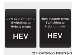
A corresponding message is displayed when the temperature of the high-voltage (hybrid) battery is too low or high. This warning message is to protect the battery and the hybrid system.
