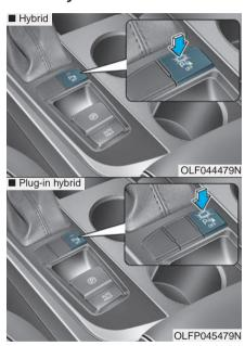
Push the button to turn off the Rear Parking Assist System. The indicator light on the button will turn on.
