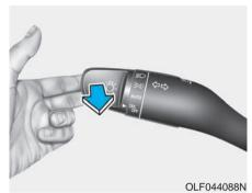
To flash the high beam headlamp, pull the lever towards you, then release the lever. The high beams will remain ON as long as you hold the lever towards you.
