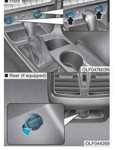
The power outlet is designed to provide power for mobile telephones or other devices designed to operate with vehicle electrical systems. The devices should draw less than 180 W with the engine running.
