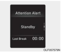
The Driver Attention Alert system enters the ready status and displays the 'Standby' screen in the following situations.
