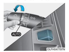
Adaptive front lighting system uses the steering angle and vehicle speed to help maximize your field of vision by swiveling and leveling the headlamp.
