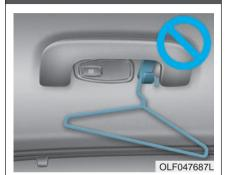
Do not hang other objects such as hangers or hard objects except clothes. Also, do not put heavy, sharp or breakable objects in the clothe pockets. In an accident or when the curtain air bag is inflated, it may cause vehicle damage or personal injury.
