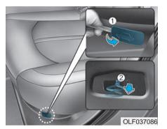
When you can not unlock the trunk due to battery discharge or other reasons, you can unlock the trunk inside the vehicle.
