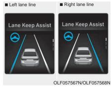
If the vehicle moves out its lane because steering torque for assistance is not enough, the line indicator of deviation direction will blink
