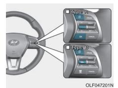
To change the trip mode, toggle the "\land , \sqrt{" switch on the steering wheel.
