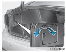
Stop/Tail lamp and Turn signal lamp (Bulb type)
