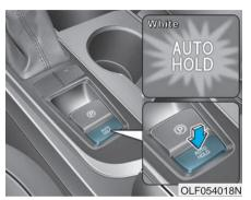
With the driver's door and the engine hood closed, fasten the driver's seat belt or depress the brake pedal and then press the [AUTO HOLD] switch. The white "AUTO HOLD" indicator will come on and the system will be in the standby position.
