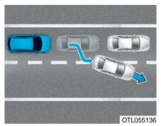
When driving in stop-and-go traffic, and a stopped vehicle in front of you merges out of the lane, the AEB system may not immediately detect the new vehicle that is now in front of you. In this case, you must maintain a safe braking distance, and if necessary, depress the brake pedal to reduce your driving speed in order to maintain a safe distance.
