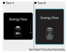
Only the engine power is used to drive the vehicle.
