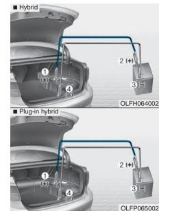
Connect the jumper cables in the exact sequence shown in the illustration. First connect one jumper cable to the red, positive (+) jumper terminal of your vehicle (1).
