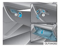
The glove box can be locked and unlocked with the mechanical key (1).
