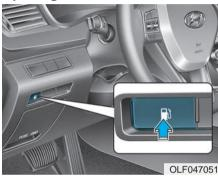
The fuel filler door must be opened from inside the vehicle by pushing the fuel filler door opener button.
