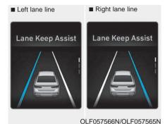
If the speed of the vehicle is over 40 mph (64 km/h) and the system detects lane markers, the color changes from gray to white.
