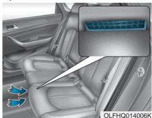
The high-voltage battery air intake is located on the bottom of the rear seats. The air intake cools down the high-voltage battery. When the high-voltage battery air intake is blocked, the high-voltage battery may be overheated and the vehicle performance may become limited and set a hybrid warning lamp. Do not obstruct the air intake with any other objects.
