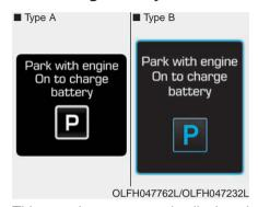
This warning message is displayed when the hybrid battery power (SOC) level is low.
