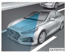
The Lane Keeping Assist System helps detect the lane markers on the road with a camera at the front windshield, and assists the driver's steering to help keep the vehicle in the lanes.
