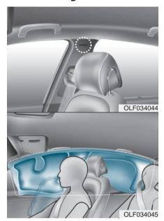
Curtain air bags are located along both sides of the roof rails above the front and rear doors.
