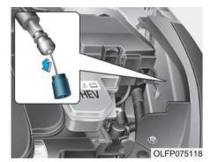
If the charging door does not open due to battery discharge, open the hood and slightly pull the emergency cable as shown above. The charging door will then open.
