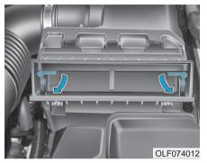
Pull down the lever to the UNLOCK position.
