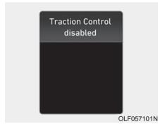
Press the ESC OFF button briefly. The ESC OFF indicator light and message will illuminate. In this state, the traction control function of ESC (engine management) is disabled, but the brake control function of ESC (braking management) still operates.
