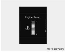
This mode displays the temperature of the engine coolant when the engine is running.
