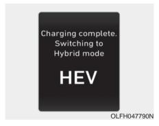
The message is displayed when the high-voltage (hybrid) battery is fully charged, and when the mode is changed to the HEV mode.
