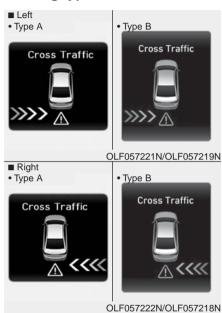
If the vehicle detected by the sensors approaches your vehicle, the warning chime will sound, the warning light on the outer side view mirror will blink and a message will appear on the LCD display.
