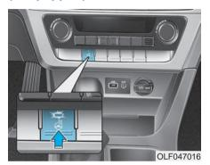
When the engine Start/Stop button is in the ON/OFF position or when the engine is running, press the heated steering wheel button to warm the steering wheel. The indicator on the button will illuminate.
