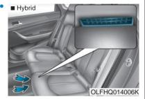
Do not put objects in the center lower part of rear seats. This could block the battery cooling duct causing battery degradation.
