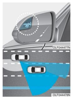
The Blind Spot Mirror (BSM) is a supplemental mirror that minimizes the driver's blind spot zone by expanding the field of view on the rear side of the vehicle. The blind spot mirror is equipped on the driver's left side view mirror.
