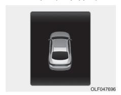
This warning is displayed when the sunroof is opened, after turning OFF the vehicle.
