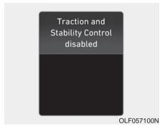
Press the ESC OFF button continuously for more than 3 seconds. The ESC OFF indicator light and message illuminates and a warning chime sounds. In this state, both the traction control function of ESC (engine management) and the brake control function of ESC (braking management) are disabled.
