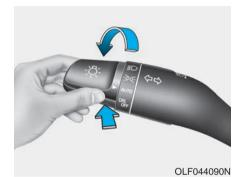
The Smart High Beam is a system that automatically adjusts the head-lamp range (switches between high beam and low beam) according to the brightness of other vehicles and road conditions.
