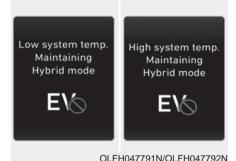
A corresponding message is displayed when the temperature of the high-voltage (hybrid) battery is too low or too high. This warning message is to protect the battery and the hybrid system.
