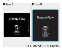
The high-voltage battery is charged up by the regenerative brake system. (Wheel → Battery)
