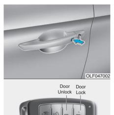
To lock the doors, press the button on the outside door handle while carrying the Smart Key with you or press the Door Lock button on the Smart Key.
