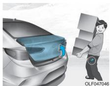
On a vehicle equipped with a smart key, the trunk can be opened with hands-free activation using the Smart Trunk system.
