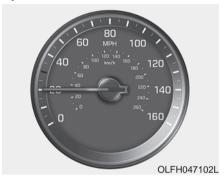
The speedometer indicates the driving speed, calibrated in miles per hour (mph) and/or kilometers per hour (km/h).
