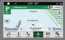
Select Destination on the screen, then select Search. You can search for a destination using a street address, partial address, city, point of interest, intersection or latitude and longitude. Once you have chosen your destination, press Start. The system uses a variety of screens and prompts to guide you to your destination.
