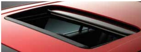
The moonroof controls are on the overhead console and have a one-touch open and close feature. To stop its movement during one-touch operation, press the control a second time. Press and release the **SLIDE** control to open or close the moonroof. Press and release the **TILT** control to vent the moonroof. The sunscreen can be manually opened or closed when the glass panel is closed.
