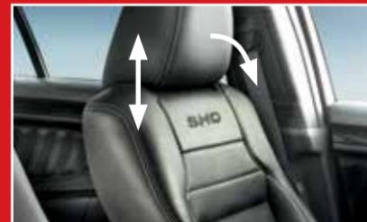
The front head restraints tilt for extra comfort. To tilt the head restraint, do the following:
