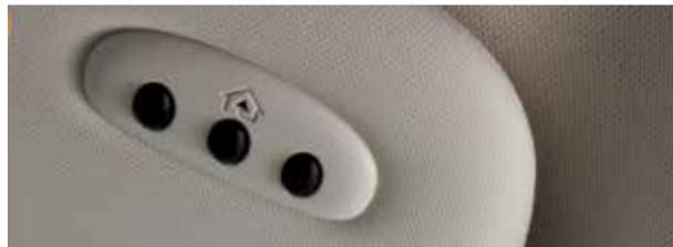
Your driver visor has a built-in wireless transmitter that replaces the common handheld garage door opener. You can program this system to security systems, entry gates and home or office lighting.
