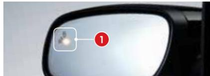
BLIS uses radar sensors to help you determine if a vehicle may be in your blind spot zone. Cross traffic alert warns you of vehicles approaching from the sides when the transmission is in reverse (R). Both systems turn on an indicator light **1** in the exterior mirror on the side of the vehicle from which the approaching vehicle is coming. Cross traffic alert also sounds tones and displays messages to warn you from which direction vehicles are approaching.
