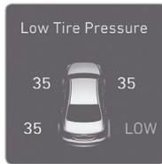
Low Tire Pressure / Tire Pressure Monitor / TPMS Malfunction Display (shown on the cluster LCD display)
