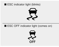
When the POWER button is pressed to the ON position, the ESC indicator light illuminates, then goes off if the ESC system is operating normally.
