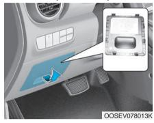
Inside the fuse/relay box cover, you can find the fuse/relay label describing fuse/relay name and capacity.
