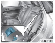
2. Make sure to insert the belt into the guide (1) and check that the seat belt is not twisted.
