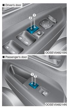
The driver side and front passenger side door armrest is equipped with a central door lock switch.
