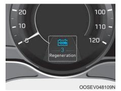
The level of regenerative braking can be selected by using the paddle shifters on the steering wheel. The level (0 to 3) is displayed in the lower portion of the cluster LCD display.
