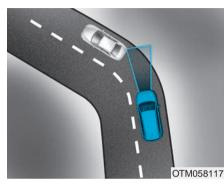
When coasting on the curve, the system may not detect the vehicle in your lane and the regenerative braking level will reduce automatically, making you feel that the vehicle is accelerating.
