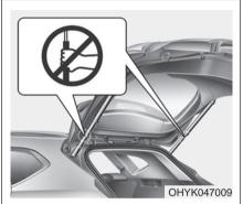
Do not hold on to or try to pull on the liftgate strut. Be aware that the deformation of the liftgate strut may cause vehicle damage and risk of injury.
