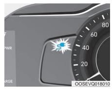
8. Check to see that the charging indicator light in the instrument cluster is illuminated. Charging has not been initiated if the charging indicator light is OFF.
