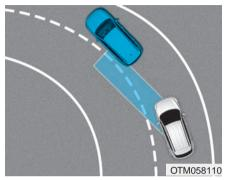
The BCW system may not operate properly when driving on a curved road. In certain instances, the system may recognize a vehicle in the same lane.
