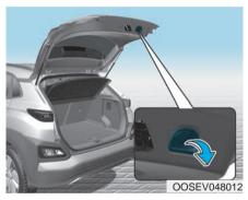
Lower the liftgate lid and press down until it locks. To be sure the liftgate lid is securely fastened, always check by trying to pull it up again without pressing the liftgate handle switch.
