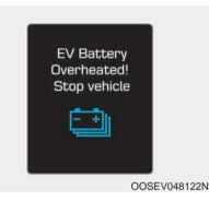
This warning message is displayed to protect battery and electric vehicle system when the high voltage battery temperature is too high.
