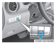
You can change the setting that locks the charging connector to the charging port on the vehicle. Change the mode using the Charging AUTO / LOCK button located on the left of the driver side dash panel.
