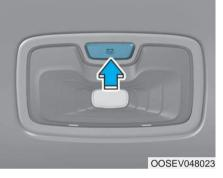
Rear Room Lamp ( 🔆 ): Press this switch to turn the rear room lamp on and off.
