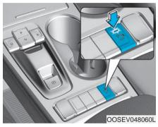
Push the button to turn OFF the Rear Parking Sensor Warning system. The indicator light on the button will turn on.
