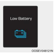
When the high voltage battery level reaches below 8%, this warning message is displayed.
