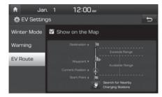
If EV route is selected, EV related information will show on the route. You can check the distance the vehicle can be driven with the current EV battery charge level % along the route.
