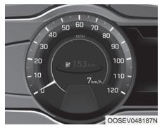
The sub speedometer is displayed on the cluster when you select 'Other features  $\rightarrow$  Speedometer subscale' in the User Settings mode. The sub speedometer is not displayed if you deselect it in the User Setting mode.
