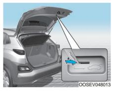
To unlock and open the liftgate manually from inside the luggage compartment, perform the following steps:
