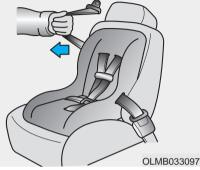
4. Pull the shoulder portion of the seat belt all the way out. When the shoulder portion of the seat belt is fully extended, it will shift the retractor to the "Automatic Locking" (child restraint) mode.
