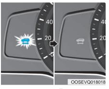
5. Check if the "🕿" indicator is turned OFF on the instrument cluster.
