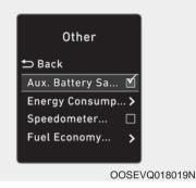
The driver can activate the Aux. Battery Saver+ function by placing the POWER button to the ON position and by selecting:
