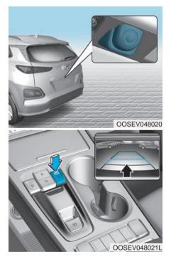
The Rear View Monitor will activate when the vehicle is in the ready ( ) mode and the gear is in the R (Reverse) position.
