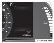
The outside temperature is shown in the lower portion of the cluster LCD display. The units may be displayed in Fahrenheit (F) or Celsius (C).
