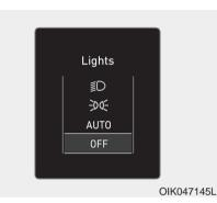
This indicator displays the exterior lights mode when selected using the headlamp control stalk.
