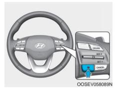
When the Smart Cruise Control system is ON, you can set and maintain the distance from the vehicle ahead of you without pressing the accelerator or brake pedal. Each time the button is pressed, the vehicle to vehicle distance changes as follows:
