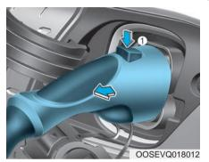
1. Hold the charging connector handle and pull it while pressing the release button (1).
