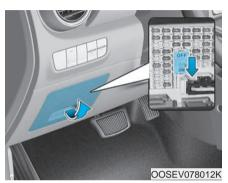
Always, place the fuse switch to the ON position.
