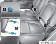
[A] : Lower Anchor Position Indicator,[B] : Lower Anchor
