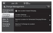
If location-based charging is selected, scheduled charging and target temperature will be activated at the location the driver has set. Also, the charging current can be selected when charged with AC charger.
