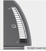
The SOC gauge shows the charging status of the high voltage battery.
