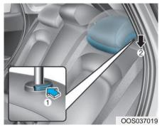
Lower the rear head restraints to the lowest position by pushing and holding the release button (1) and pushing down on the headrest (2).
