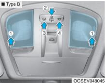
Front Map Lamp (1) : Press either of these lenses to turn the map lamp on or off. This light produces a spot beam for convenient use as a map lamp at night or as a personal lamp for the driver and the front passenger.
