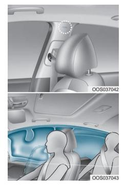
Curtain air bags are located along both sides of the roof rails above the front and rear doors. They are designed to help protect the heads of the front seat occupants and the rear outboard seat occupants in certain side impact collisions.
