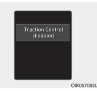
Press the ESC OFF button briefly. The ESC OFF indicator light and message "Traction Control disabled" will illuminate. In this state, the traction control function of ESC is disabled, but the brake control function of ESC still operates.
