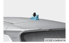
The shark fin antenna will receive the AM, FM broadcast signals and transmit data.
