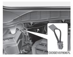
In case of emergency, cut the service interlock connector cable to isolate the high voltage of the battery.
