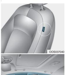
Your vehicle is equipped with a side air bag in each front seat.
