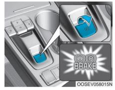
To apply the EPB (Electronic Parking Brake):
