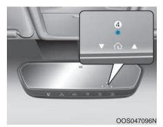
4. Press the Original Transmitter (OT) button until the indicator (4) is turned continuously ON or flashes in Green for approximately 10 seconds and it indicates the programing is completed.
