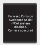
However, the FCA may not properly operate in an area (e.g. open terrain), where any substances are not detected or the camera is blocked with dirt, snow or debris after turning ON the vehicle.
