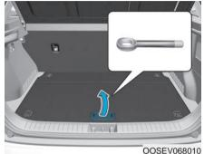
1. Open the liftgate, and remove the towing hook from the tool case.
