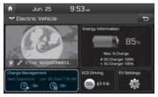
Select 'EV  $\rightarrow$  Charge Management' on the screen. You can set the date and time of when to charge the battery, climate control temperature, location-based charging options and other various functions.
