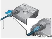
2. Connect the filling hose (3) directly into the compressor.
