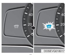
8. When the "🕿" indicator is ON, you can drive the vehicle.
