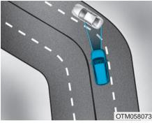
Your vehicle speed can be reduced due to a vehicle in the adjacent lane. Apply the accelerator pedal and select the appropriate set speed. Check to be sure that the road conditions permit safe operation of the Smart Cruise Control.
