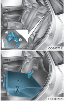
4. Remove the belt from the guide (1) and pull up the seatback folding lever (2), then fold the seat toward the front of the vehicle.
