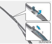
2. Lift up the wiper blade clip (1). Then pull down the blade assembly and remove it (2).
