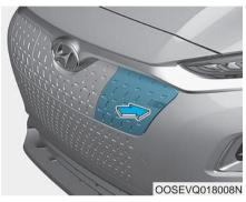
The charging door is located on the front of the vehicle and can be opened when the vehicle doors are unlocked.
