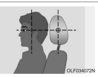
Adjust the head restraints so the middle of the head restraints is at the same height as the height of the top of the eyes.
