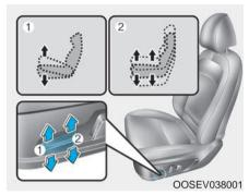
Seat cushion tilt (1, if equipped) To change the angle of the front part of the seat cushion:
