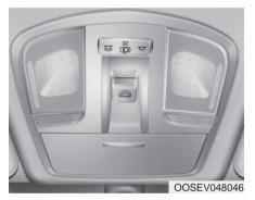
The sunroof can be opened, closed, or tilted when the POWER button is in the ON position.
