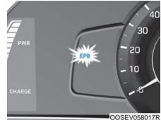
This warning light illuminates if the POWER button is changed to the ON position and goes off in approximately 3 seconds if the system is operating normally.
