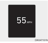
This digital speedometer display shows the speed of the vehicle.
