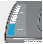
The Power/Charge gauge shows the energy consumption rate of the vehicle and the charge/discharge status of the regenerative brakes.
