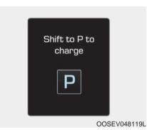
This message is displayed if you connect the charging cable without the gear in the P (Park) position. Shift to P (Park) before connecting the charging cable.
