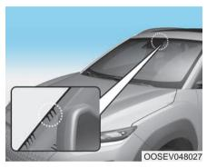
Auto defogging helps reduce the possibility of fogging up the inside of the windshield by automatically sensing the moisture on inside the windshield.
