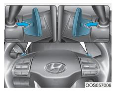
The paddle shifter is used to adjust the regenerative braking level from 0 to 3 during decelerating or braking.
