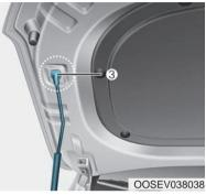
4. Pull out the support rod and hold the hood open with the support rod (3).
