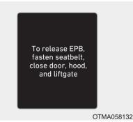
To release EPB, fasten seatbelt, close door, hood and liftgate
