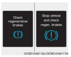
This warning message is displayed when the regenerative brake system does not work properly.
