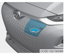
Unlock the vehicle before opening the charging door. From the outside the vehicle, push on the charging door in the area indicated by the arrow to open the door.
