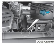
If for some reason the charging connector fails to disconnect normally, the connector may be released manually using the Charging Connector Manual Release. Open the hood and slightly pull the manual release shown in the figure. The charging connector can then be disconnected.
