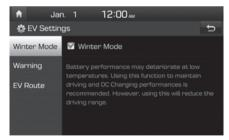
In cold climates and during winter months, electric vehicle range may reduce and charging times may increase. This is primarily due to reduced performance of the EV battery when exposed to cold temperatures.
