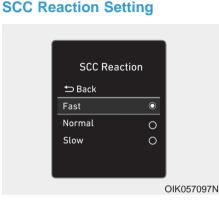
The sensitivity of vehicle speed when following the front vehicle to maintain the set distance can be adjusted. Go to the 'User Settings  $\rightarrow$  Driver Assistance  $\rightarrow$  SCC Reaction  $\rightarrow$  Fast/Normal/Slow' on the LCD display. You may select one of the three stages you prefer.
