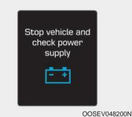
This warning message is displayed when a failure occurs in the power supply system.
