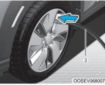
4. Unscrew the valve cap from the valve of the defective wheel and screw the filling hose (3) of the sealant bottle onto the valve.
