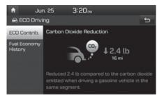
The CO2 reduction display allows you to monitor the benefits of reduced greenhouse gas emissions of your EV relative to a conventional gasoline vehicle. While driving your vehicle, the display estimates the amount of reduced CO2 that would have been emitted from tailpipe emissions of a conventional vehicle.
