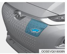
5. Unlock the vehicle before opening the charging door. Push on the charging door in the area indicated by the arrow to open the door.
