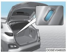
The luggage compartment lamp comes on when the liftgate is opened.
