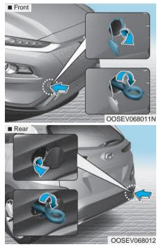
2. Remove the hole cover by pressing the lower part of the cover on the front or rear bumper.
