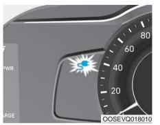
7. Check to see that the charging indicator light in the instrument cluster is illuminated. Charging has not been initiated if the charging indicator light is OFF.
