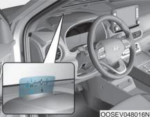
The Head-Up Display is an optional feature that allows the driver to view information projected onto a transparent screen while still keeping your eves safely on the road ahead while driving.
