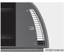
The SOC gauge shows the charging status of the high voltage battery.
