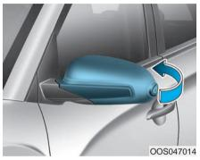
To fold the side view mirrors, grasp the housing of the mirror and then fold it inwards.
