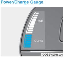
The Power/Charge gauge shows the energy consumption rate of the vehicle and the charge/discharge status of the regenerative brakes.
