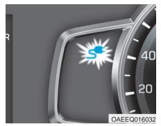
10. Check to see that the charging indicator light in the instrument cluster is illuminated. Charging has not been initiated if the charging indicator light is OFF.
