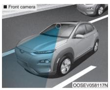
In order for the FCA system to operate properly, always make sure the camera is clean and free of dirt, snow, and debris. Dirt, snow, or foreign substances on the surface may adversely affect the sensing performance of the sensor.
