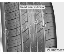
If the tire is worn evenly, a tread wear indicator will appear as a solid band across the tread. This shows there is less than 1/16 inch (1.6 mm) of tread left on the tire. Replace the tire when this happens.
