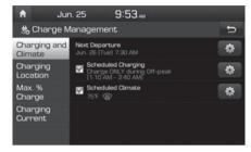
You can set the date and time of when to charge the battery and the climate control temperature. Also, you may select the time to start charging using the off-peak hours setting.
