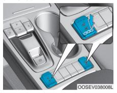
The ventilated front seats are provided to cool the front seats by blowing air through small vent holes on the surface of the seat cushions and seatbacks.
