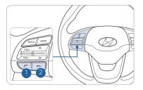
1. Press the SETUP button on the head unit or the CALL button on the steering wheel.
