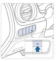
The Lane Keeping Assist System detects lane markers on the road with a camera and assists the driver's steering to help keep the vehicle between lanes. The system operates when the vehicle speed is above 40 mph
