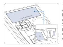
There is a wireless cellular phone charging system in front of the cup holders. The system operates with all doors closed, and the Start/ Stop button in the ACC/ON/START position. Wireless charging system can be disabled in the instrument cluster settings menu.
