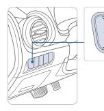
Press the illumination control button to adjust the instrument cluster illumination brightness.
