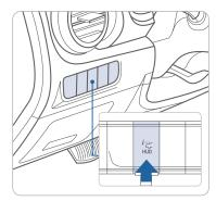
To activate the Heads-Up Display, press the HUD button on the dash panel located on the left-hand side of the driver.
