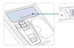
Use the Aux input jack to connect an external audio device. Use the media USB port to connect a USB device with music files or to access features on your smartphone using Apple CarPlay or Android Auto phone projection.
