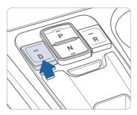
Select gear positions by pressing the shift button. The gear position is displayed in the instrument cluster.
