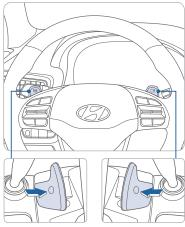
The level of regenerative braking can be selected by using the paddle shifters on the steering wheel. The level (0 to 3) is displayed in the lower portion of the cluster LCD display.
