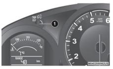
**Odometer/Trip Reset Button**
