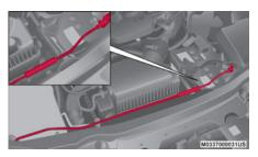
**Inserting Support Rod Into Hole**
