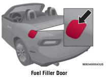
The fuel filler door operates in conjunction with the door locking/unlocking mechanism.
