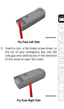
. Separate the key fob case, then remove the battery.
