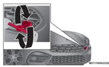
Abarth Installing Front Towing Eye
