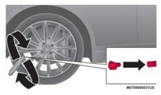
**Turn Valve Core Clockwise To Reinstall**
