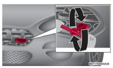
**Installing Front Towing Eye**
