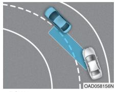
BCW system may not operate properly when driving on a curved road. In certain instances the system may recognize a vehicle in the same lane.
