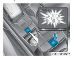
With the driver's door and hood closed, fasten the driver's seat belt or depress the brake pedal and then press the [AUTO HOLD] switch. The white AUTO HOLD indicator will come on and the system will be in the standby position.
