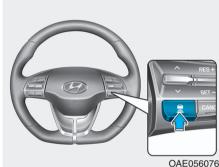
When Smart Cruise Control system is ON, you can set and maintain the distance from the vehicle ahead of you without pressing the accelerator or brake pedal.
