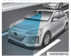
Lane Following Assist system helps detect lane markers on the road with a front view camera at the front windshield, and assists the driver's steering to help keep the vehicle between lanes.
