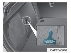
If the charging door does not open due to battery discharge and failure of the electric wires, open the liftgate and slightly pull the emergency cable as shown above. The charging door will then open.
