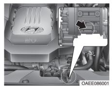
The motor number is stamped on the motor block as shown in the drawing. The motor number can be seen from under the vehicle.
