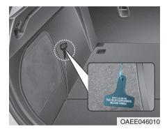
If the charging door does not open due to battery discharge and failure of the electric wires, open the liftgate and slightly pull the emergency cable as shown above. The charging door will then open.
