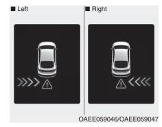
If the vehicle detected by the sensors approaches from the rear left/right side of your vehicle, the warning chime will sound, the warning light on the outside rearview mirror will blink and a message will appear on the LCD display. If the rear view monitor system is in activation, a message will also appear on the audio or infotainment system screen.
