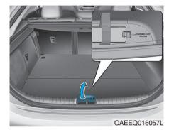
If the charging connector does not disconnect due to battery discharge and failure of the electric wires, open the liftgate and slightly pull the emergency cable. The charging connector will then disconnect.
