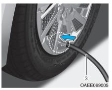
Unscrew the valve cap from the valve of the flat tire and screw the filling hose (3) of the sealant bottle onto the valve.
