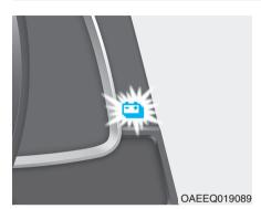
When there are 4~5 gauge bars (near the "L (Low)" area) on the SOC gauge, the warning lamp turns ON to alert you of the battery level.
