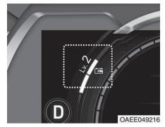
The selected regenerative braking rate is displayed on the instrument cluster.
