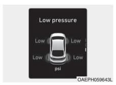
When the tire pressure monitoring system warning indicators are illuminated and the warning message is displayed on the cluster LCD display, one or more of your tires is significantly under-inflated. The LCD position indicator will indicate which tire is significantly under-inflated by illuminating the corresponding position light.
