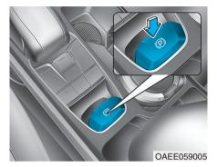
To release EPB (Electronic Parking Brake):
