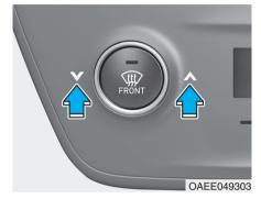
Press the button to increase/ decrease the fan temperature and airflow.
