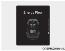
Only the motor power is used to drive the vehicle. (Battery → Wheel)
