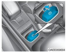
To apply the EPB (Electronic Parking Brake):
