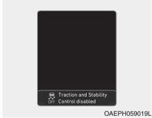
Press and hold the ESC OFF button continuously for more than 3 seconds. The ESC OFF indicator light And/or message "Traction & Stability Control disabled" illuminates and a warning chime sounds. In this state, both the traction control function of ESC and the brake control function of ESC are disabled.
