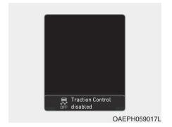
Press the ESC OFF button briefly. The ESC OFF indicator light And/or message "Traction Control disabled" will illuminate. In this state, the traction control function of ESC is disabled, but the brake control function of ESC still operates.
