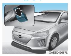
Auto defogging system reduces the possibility of fogging up the inside of the windshield by automatically sensing the moisture of inside the windshield.
