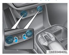
The power outlet is designed to provide power for mobile telephones or other devices designed to operate with vehicle electrical systems. The devices should draw less than 180 W (Watts) with the vehicle in the ready () mode.
