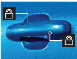
To unlock, place your hand between the back of the front door handle and the vehicle for a brief period and then pull on the door handle, being careful to not touch the lock sensor at the same time or pull the door handle too quickly.
