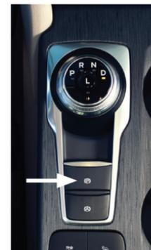
To release the electric parking brake manually, switch the ignition on, press the brake pedal and then press the switch down. The brake system warning lamp turns off. Your vehicle automatically releases the parking brake when the driver door is closed, the accelerator pedal is pressed and no faults are detected in the parking brake system.
