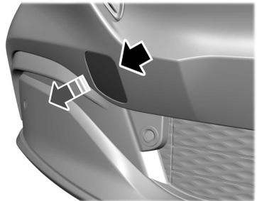
2. Remove the cover at the front of your vehicle below the headlight. Press firmly on the top right of the covers edge, then pull the raised section on the bottom left toward you.
