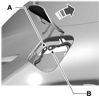
3. Pull both wires out of the opening to reveal both terminals.
