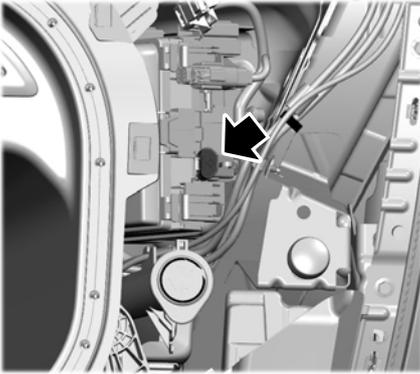
1. Connect the positive (+) jumper cable to the positive (+) jump point of the discharged battery vehicle.
