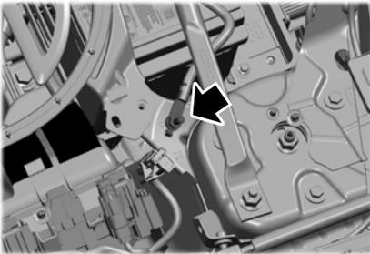
4. Make the final connection of the negative (-) jumper cable to the negative (-) ground point of the discharged battery vehicle.
