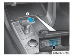
You can use an AUX or USB cable to connect audio devices to the vehicle AUX or USB port.
