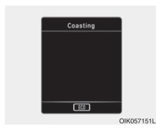
When the ECO Coasting function is activated 'Coasting' illuminates on the top of the instrument cluster.
