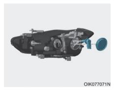
Disconnect the bulb socket-connector.
