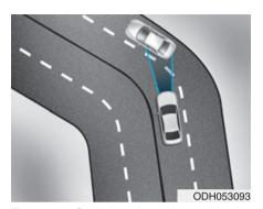
Forward Collision-Avoidance Assist system may recognize a vehicle or pedestrian or cyclist in the next lane or outside the lane when driving on a curved road.
