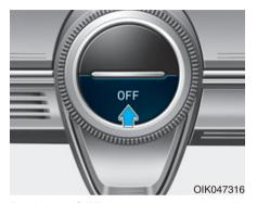
Push the OFF button to turn the climate control system off. You can still operate the mode and air intake buttons as long as the Engine Start/Stop button is in the ON position.
