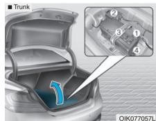
When replacing the battery, disconnect the negative (-) cable (1) and remove the positive (+) battery fuse box (2). Remove the trunk panel and spare wheel. Place the spare wheel on the floor with the finished side up so as not to damage. Then remove the spare wheel bracket (3) followed by the battery hold down mounting bracket (4).
