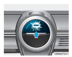
Adjusting the driver and passenger side temperature equally
