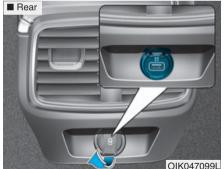
The USB charger is designed to recharge batteries of small size electrical devices using a USB cable.
