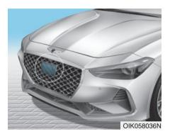
The Smart Cruise Control uses a sensor to detect distance to the vehicle ahead.
