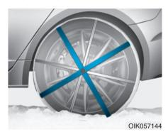
Since the sidewalls on some radial tires are thinner than other types of tires, they may be damaged by mounting certain types of tire chains on them. Do not mount tire chains on vehicles equipped with aluminum wheels; if unavoidable use AutoSock® (fabric snow chain or similar). Install the tire chain after reviewing the instructions provided with the tire chains. Damage to your vehicle caused by improper tire chain use is not covered by your vehicle manufacturer's warranty.
