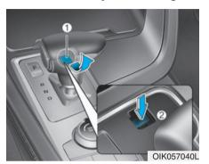
You cannot move the shift lever, when the battery is discharged.
