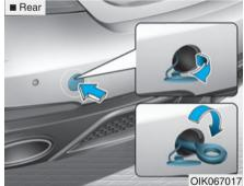
2. Remove the hole cover pressing the lower part of the cover on the front or rear bumper.
