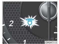
If the AFS malfunction indicator comes on, the AFS is not working properly. Drive to the nearest safe location and restart the engine. If the indicator continuously remains on, have the system checked by an authorized retailer of Genesis Branded products.
