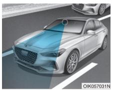
The Lane Keeping Assist (LKA) system helps detect lane markers on the road with a front view camera at the front windshield, and assists the driver's steering to help keep the vehicle between lanes.
