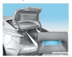
The trunk lamp comes on when the trunk is opened.
