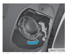
3. Remove the bulb cover by turning it counterclockwise.
