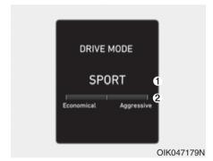
The drive mode selected by the driver (1) and the driving style gauge (2) showing the driver's driving style are displayed on the screen.
