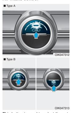
This button is used to select the outside (fresh) air position or recirculated air position.
