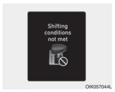
The message appears on the LCD display when engine rpm is too high, or when driving speed is too fast to shift the gear.
