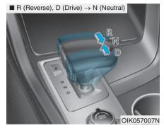
The wheels and transmission are not engaged.
