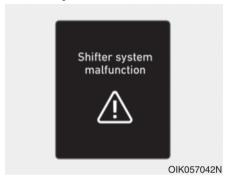
The message appears on the LCD display when the transmission or the shift lever does not properly operate in the P (Park) position.
