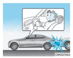
Front air bags are not designed to inflate in rear collisions, because occupants are moved backward by the force of the impact. In this case, inflated air bags would not provide any additional benefit.
