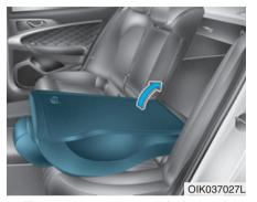
To use the rear seat, lift and unfold the seatback to the upright position. Push the seatback firmly until it clicks into place. Make sure the seatback is locked in place.
