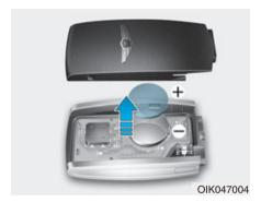
Battery Type: CR2032 To replace the battery:
