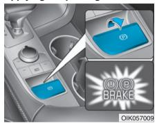
To apply the EPB (Electronic Parking Brake):
