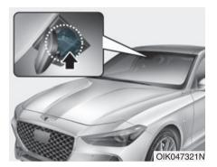
Auto defogging helps reduce the possibility of fogging up the inside of the windshield by automatically sensing the moisture on inside the windshield. The auto defogging system operates when the heater or air conditioning is on.
