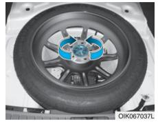
Turn the winged hold down bolt counterclockwise to remove the spare tire.
