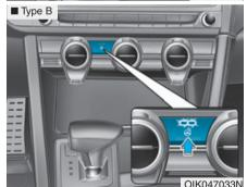
When the Engine Start/Stop button is in the ON position, press the heated steering wheel switch to warm the steering wheel.  Each time you push the switch, the temperature setting changes as follows:
