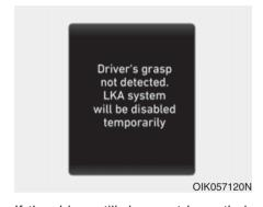
If the driver still does not have their hands on the steering wheel after the message "Keep hands on steering wheel", the system will not control the steering wheel and warn the driver only when the driver crosses the
