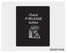
The message appears on the LCD display when there is problem with the P RELEASE button.
