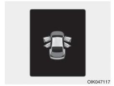
This warning is displayed if any door or the hood or the trunk is left open. The warning will indicate which door is open in the display.
