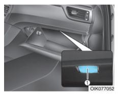
If the glove box lamp (LED) (1) does not operate, have the system be checked by an authorized retailer of Genesis Branded products.
