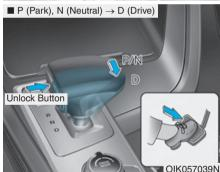
To shift into D (Drive), depress the brake pedal and press the UNLOCK button on the shift lever. Move the shift lever rearward.
