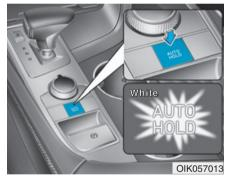
With the driver's door and engine hood closed, fasten the driver's seat belt or depress the brake pedal and then press the [AUTO HOLD] switch. The white AUTO HOLD indicator will come on and the system will be in the standby position.
