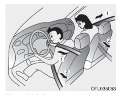
Your vehicle is equipped with driver's and front passenger's Pre-tensioner Seat Belts (Retractor Pretensioner and Emergency Fastening Device System). The purpose of the pre-tensioner is to make sure the seat belts fit tightly against the occupant's body in certain frontal or side collision(s). The Emergency Fastening Device System may be activated in certain crashes where the frontal or side collision(s) is severe enough, together with the air bags.
