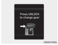
The message appears on the LCD display when the UNLOCK button is not pressed while shifting the gear. Press the UNLOCK button and then shift the gear.
