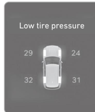
To access the TPMS menu within the LCD display, press the Driving Assist mode button on the steering wheel to display tire pressure.
