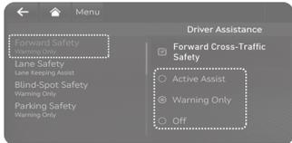
Forward Collision-Avoidance Assist designed to detect and monitor the vehicle ahead and warn the driver if a collision is imminent. On vehicles equipped with both front view camera and front radar sensor, a pedestrian or a cyclist detection is also available.
