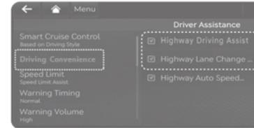
Highway Driving Assist helps maintain a set distance and speed from the vehicle ahead when driving on a highway and helps center the vehicle in the lane while driving, even through a curve.
