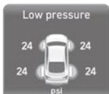
Low Tire Pressure / Tire Pressure Monitor / TPMS Malfunction Display (shown on the cluster LCD display)
