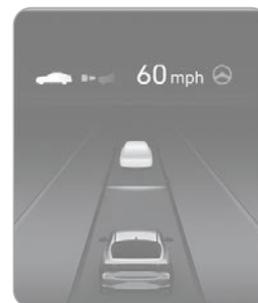
Press the Vehicle distance button to set and maintain the vehicle distance without pressing the accelerator or brake pedal. The vehicle distance will automatically activate previous setting value when you activate SCC.
