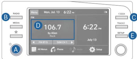
Press POWER button **A** to turn radio on.
