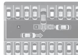
RCCA uses radar sensors to monitor approaching vehicles to the left or right while your vehicle is in reverse. If the risk of collision is detected while the RCCW is generated, brake is controlled. The instrument cluster will inform the driver of the brake control. If Rear View Monitor is in activation, a message will also appear on the audio or AVN screen.
