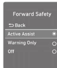
Forward Collision-Avoidance Assist is designed to detect and monitor the vehicle ahead and warn the driver if a collision is imminent. This feature also allows pedestrian detection.
