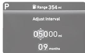
Service Interval > Enable Service Interval > Set/Adjust Interval.
