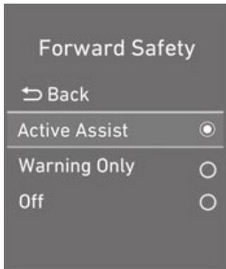
Forward Collision-Avoidance Assist is designed to help detect and monitor the vehicle ahead or help detect a pedestrian or cyclist in the roadway and warn the driver that a collision is imminent with a warning message and an audible warning, and if necessary, apply emergency braking.
