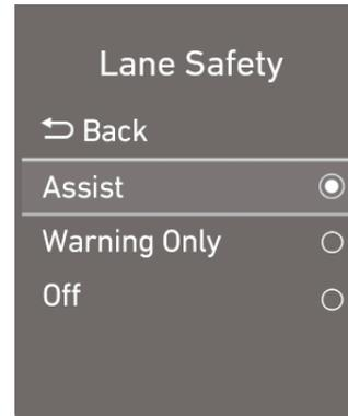
LKAS operates only when the vehicle speed is above 40 mph and when the LKAS indicator is green displayed in the instrument cluster. LKAS will not operate properly if the lane line is not clear, sharp bend in the road, or in heavy fog. Refer to the Owner's Manual for more detailed information.
