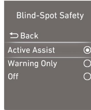
Blind-Spot Collision-Avoidance Assist (BCA) system is designed to help detect and monitor approaching vehicles in the driver's blind spot area and warn the driver of a possible collision with a warning message and audible warning. In addition, if there is a risk of collision when changing lanes or driving forward out of a parking space, the system will help avoid a collision by applying the brake.
