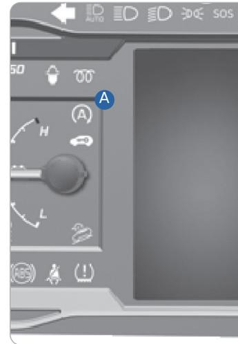
The ISG system will automatically shut off the engine when the vehicle is at a standstill (i.e. red stop light, stop sign, and traffic jam) to increase vehicle’s fuel economy. The auto stop indicator **A** will illuminate in Green on the instrument cluster when activated. To restart the engine in auto stop mode, release the brake pedal and press on the accelerator. The auto stop indicator goes OFF on the instrument cluster once the engine is restarted.
