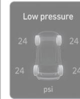
Low Tire Pressure / Tire Pressure Monitor / TPMS Malfunction Display (shown on the cluster LCD display)
