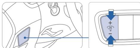
Press + or - to adjust the illumination brightness of the instrument cluster.
