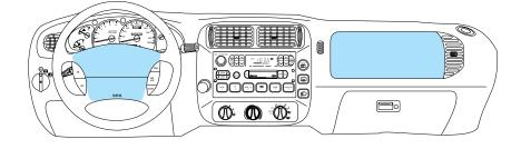
The Explorer incorporates dual standard (driver and passenger) air bag supplemental restraint systems.
