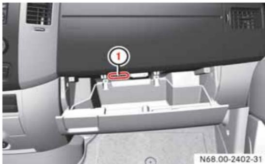
① To switch the air supply on / off
