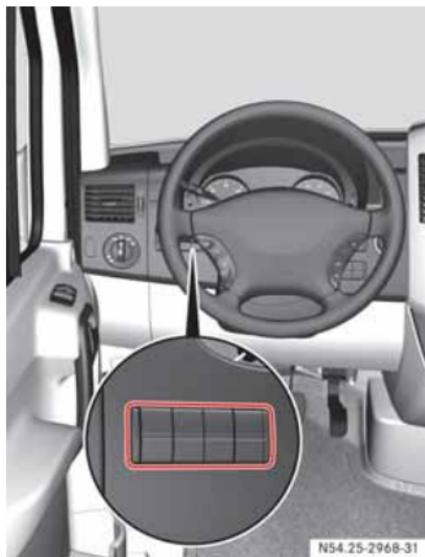
Switch unit between the light switch and the steering wheel
