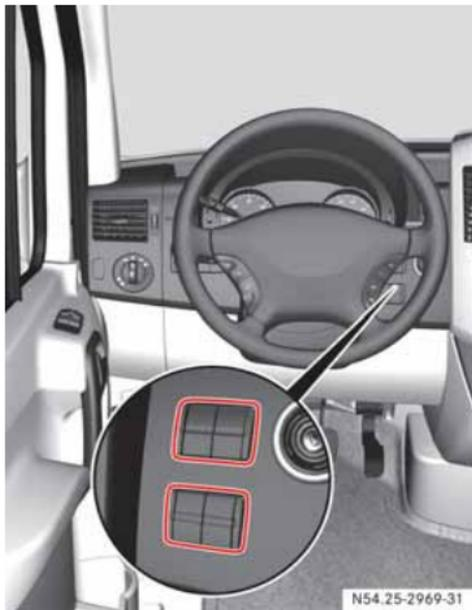
Switch unit between the steering wheel and the ignition lock
