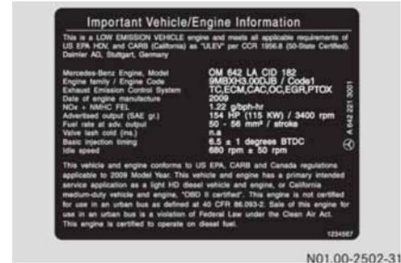
**Example emission control information label for diesel engines (U.S. vehicles)**
