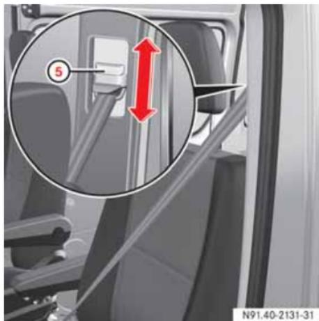
**Belt sash guide with height adjustment**
