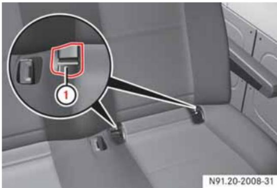
① Securing rings - LATCH type anchors
