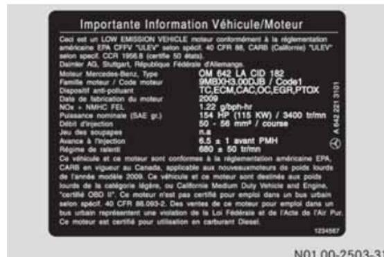
Example emission control information label for diesel engines (Canada vehicles)
