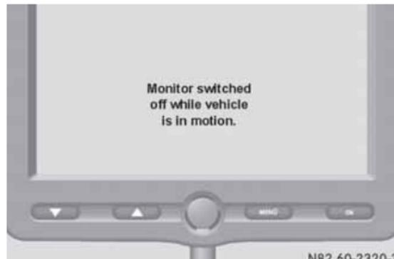
If the speed falls below 5 mph (8 km/h), the monitor switches on again.
