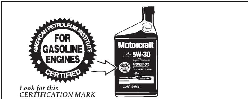
Use SAE 5W-30 motor oil certified for gasoline engines by the American Petroleum Institute.
