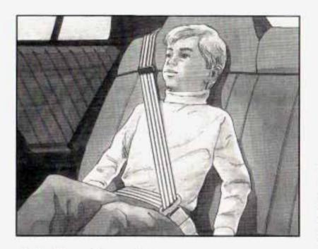
Buckle, position and release the safety belt as described in Rear Seat Passengers on page 1-24. Make sure that the shoulder belt crosses the shoulder To remove and store the comfort guides, squeeze the belt edges together so that you can take them out of the guides. Pull the guide upward to expose its storage clip, and then slide the guide onto the clip. Turn the guide and clip inward and in between the seatback and the interior body, leaving only the loop of the elastic cord exposed.
