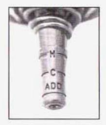
When the engine compartment is hot, the level should be at the H (hot) mark. When it's cold, the level should be at the C (cold) mark. If the fluid is at the ADD mark, you should add fluid.
