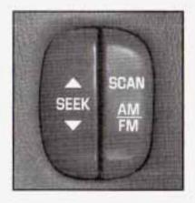
$\triangle$  **SEEK**  $\nabla$ : Press the up or the down arrow to seek to the next or the previous radio station.
