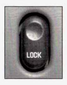
Your vehicle is equipped with front power door lock switches. Press a power door lock switch to lock or unlock all doors.
