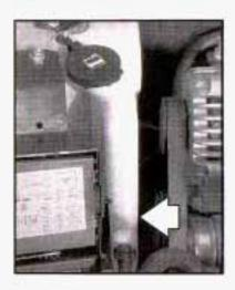
The vehicle must be on a level surface. When your engine is cold, the coolant level should be at the COLD mark or a little higher. When your engine is warm, the level should be up to the HOT mark or a little higher.
