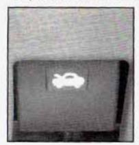
Pull the handle inside the vehicle, located just below the instrument panel and to the left of the steering column.
