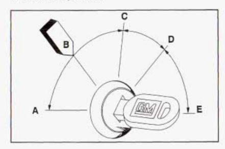
A (ACCESSORY): This position lets you use the radio and windshield wipers when the engine is off. To use ACCESSORY, push in the key and turn it toward you. Your steering wheel will stay locked.
