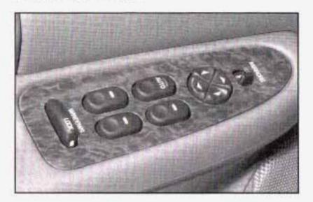
The switches on the driver's door armrest can be used to control each of the windows when the ignition is on. In addition, each passenger's door has a window switch.
