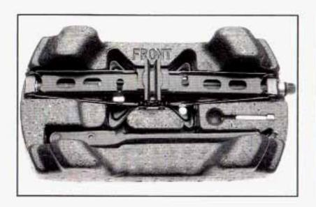
Turn the nut holding the jack counterclockwise and remove it. Then remove the jack and wrench.
