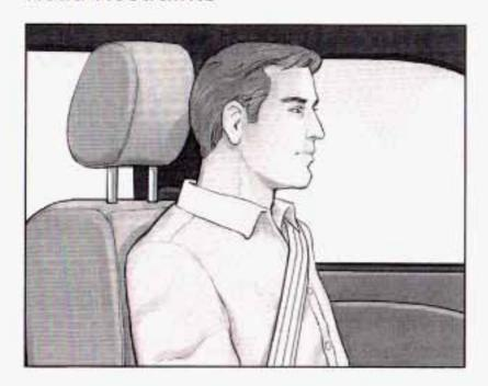
Adjust your head restraint so that the top of the restraint is closest to the top of your head. This position reduces the chance of a neck injury in a crash.
