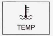
This light tells you that your engine coolant has overheated or your radiator cooling fan is not working.
