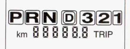
The graphic shown above is displayed on your instrument panel cluster and will indicate the gear your vehicle is in when you move.
