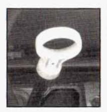
The engine oil dipstick handle is the yellow loop located near the front of the engine. See Engine Compartment Overview on page 5-12 for more information on location.
