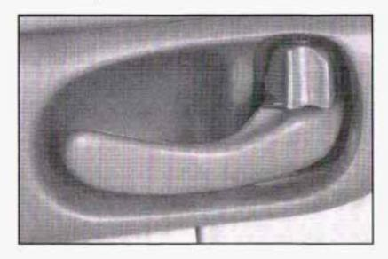
To lock the door from the inside, push the manual lock lever forward. To unlock the door, push the lever rearward.
