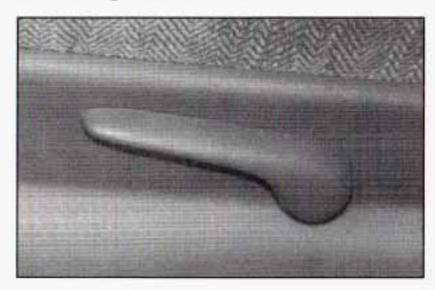
Lift the lever located on the outboard side of the seat to release the seatback, then move the seatback to where you want it. Release the lever to lock the seatback in place. Pull up on the lever without pushing on the seatback and the seatback will move forward.
