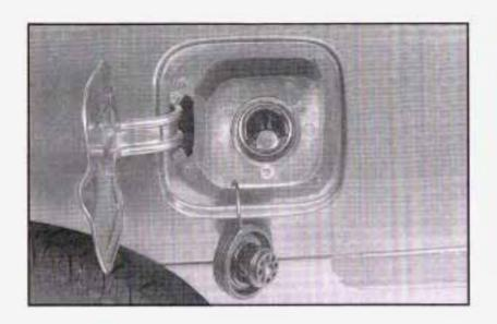
While refueling, let the fuel cap hang by the tether below the fuel fill opening.
