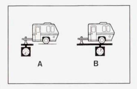
If you're using a weight-carrying hitch or a weight-distributing hitch, the trailer tongue (A) should weigh 10–15 percent of the total loaded trailer weight (B).
