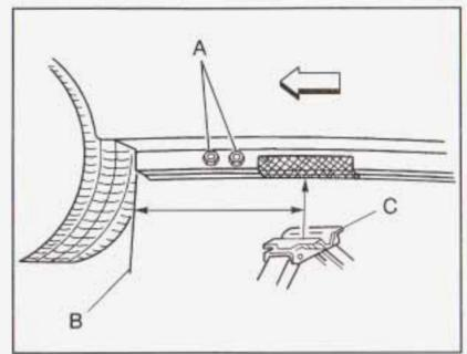
For jacking at the vehicle's front location, put the jack lift head (C) about 6 inches (15 cm) from the rear edge of the front wheel opening (B) or just behind the two bolts (A) as shown.
