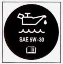
The engine oil fill cap is located toward the front of the engine near the engine oil dipstick handle. See Engine Compartment Overview on page 5-12 for more information on location.
