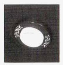
Press the button located inside of the glove box door to release the trunk from inside the vehicle. The shift lever must be in PARK (P) for the remote trunk release button to work.
