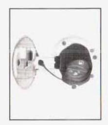
The fuel cap is located behind a hinged door on the driver's side of your vehicle.
