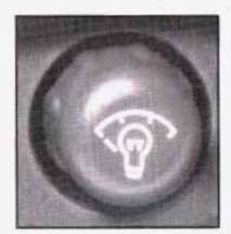
Press this knob located next to the exterior lamps knob to extend and turn it to make your instrument panel brighter. Turn the knob all the way up to turn on the interior lamps. Press the knob back into its stored position.
