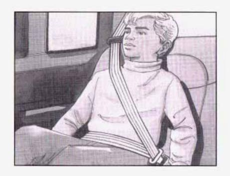
Buckle, position and release the safety belt as described in Rear Seat Passengers on page 1-27. Make sure that the shoulder belt crosses the shoulder.
