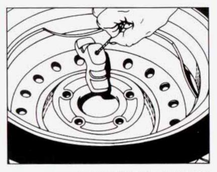
When the tire has been lowered, pull the tire toward you so you can reach the tire retainer and pull it up through the wheel opening.
