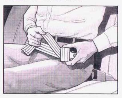
When you sit in a center seating position in the third, fourth or fifth row, you have a lap safety belt, which has no retractor. To make the belt longer, tilt the latch plate and pull it along the belt.
