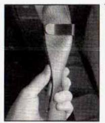
For the first rear seat, stow the safety belt latch by attaching the clip on the safety belt latch to the trim just inside the side door. For the remaining rear seats, stow the safety belt latch plate on the clip at the window trim.
