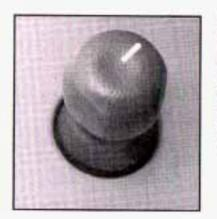
Select the mirror you want to move by turning the knob clockwise to adjust the passenger's side mirror and counterclockwise to adjust the driver's side mirror. The center position is neutral.
