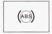
If there's a problem with the anti-lock brake system, this warning light will stay on. See Anti-Lock Brake System Warning Light on page 3-32.
