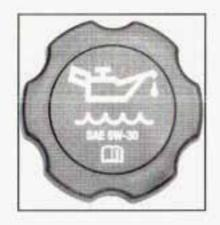
The engine oil filler cap is located between the coolant recovery tank and the engine air cleaner/filter. See Engine Compartment Overview on page 5-12 for more information on location.
