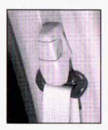
To move it down, pull on the center adjuster control labeled PULL. You can move the adjuster up just by pushing up on the shoulder belt guide. After you move the adjuster to where you want it, try to move it down without pushing in to make sure it has locked into position.
