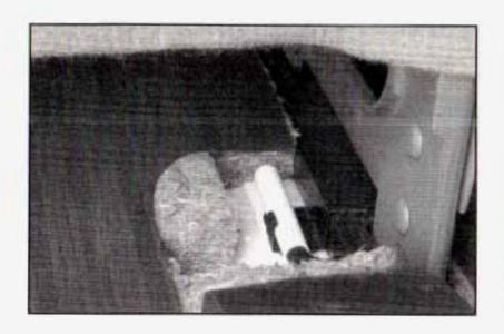
Push the pin with the white handle marked "R" down until it is in the retaining clip.
