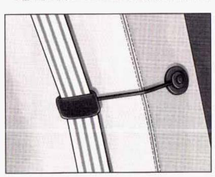
Be sure the belt is not twisted and it lies flat. The elastic cord must be under the belt and the guide on top.
