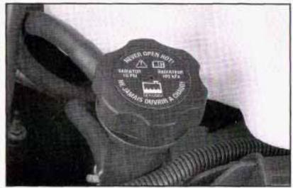
Then replace the pressure cap. At any time during this procedure if coolant begins to flow out of the filler neck, reinstall the pressure cap.
