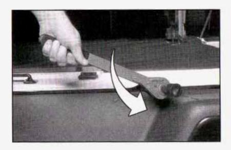
Turn the ratchet counterclockwise to lower the spare tire to the ground. If the spare tire does not lower to the ground, the secondary latch is engaged causing the tire not to lower. See "Secondary Latch System" later in this section.
