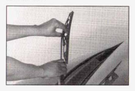
Replacement blades come in different types and are removed in different ways. To remove the type with a release clip, do the following:
