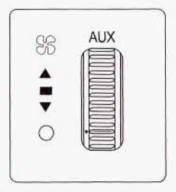
AUX (Auxiliary Heating System): The thumbwheel for this system is located to the right of the audio system.
