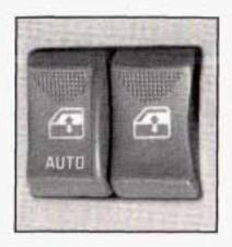
If you have power windows, the controls are located on each of the side doors. The driver's door has a switch for the passenger window as well. Your power windows will work when the ignition has been turned to RUN or ACCESSORY, or when Retained Accessory Power (RAP) is active. See Ignition Positions on page 2-20.
