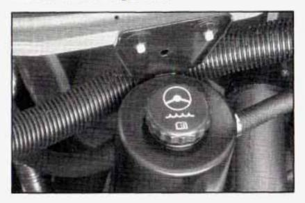
The power steering fluid reservoir is located in the engine compartment on the driver's side of the vehicle.
