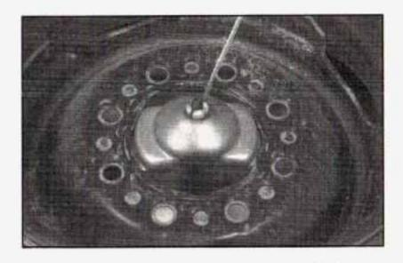
Pull the retaining bar through the center of the wheel, making sure it is properly attached.
