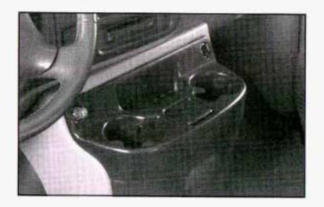
Your front storage compartment is at the center of the instrument panel extension, by the floor. To open the compartment, press down on the inside portion of the handle. The compartment will open automatically.
