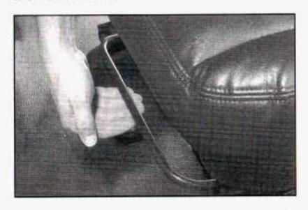
The bucket seats can be adjusted forward or rearward with the lever located at the front of the seat.
