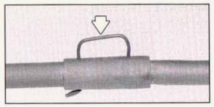
Connect the jack handle (C) and jack handle extension (B) together and press the retention clip (arrow) so it engages.
