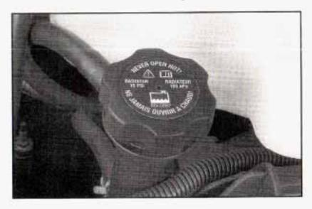
The radiator pressure cap is located near the center of the engine compartment.
