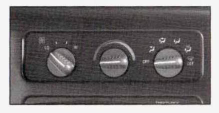
Turn the right knob clockwise or counterclockwise to direct the airflow inside of your vehicle.
