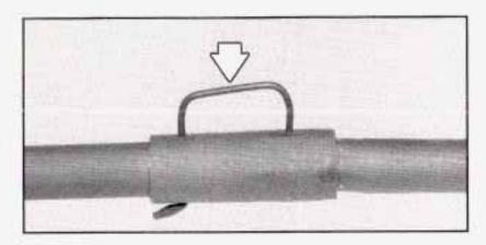
Connect the jack handle (B) and jack handle extension (C) together and press the retention clip (arrow) so it engages.
