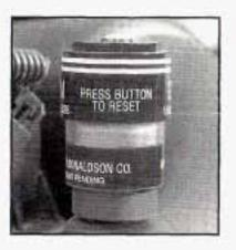
Your vehicle may have this feature. The engine air cleaner/filter assembly has an indicator that lets you know when the air filter is dirty and needs to be serviced.
