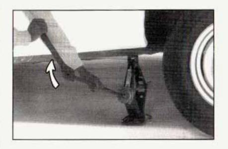
Raise the vehicle by turning the ratchet clockwise.
