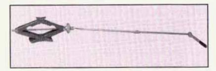
Attach the jack handle/jack handle extension to the jack and slide the ratchet with the UP mark facing you onto the end of the jack handle extension so your set-up looks like the picture above.
