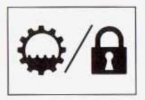
The transmission dipstick is located near the center of the engine compartment and will be labeled with this graphic shown. See Engine Compartment Overview on page 5-12 for more information on location.
