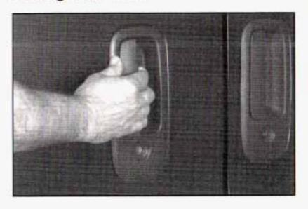
To open the sliding side door from outside, pull the handle toward the rear of the vehicle. Then, slide the door open.
