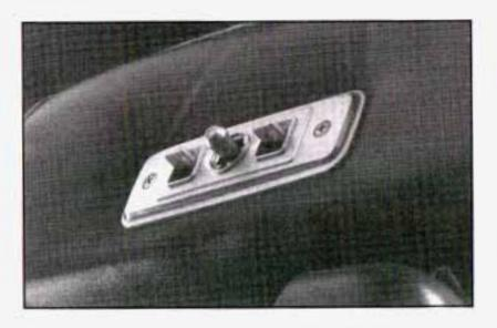
If your vehicle has a power seat on the driver's or passenger's side, you can adjust it with these controls located at the front center of the seat cushion.
