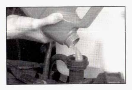
Fill the radiator with the proper DEX-COOL<sup>®</sup>
