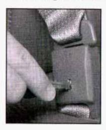
Disconnect the quick release latch plates for the lap shoulder belts on the bench seat to be removed. To do this, press the tip of a key into the release hole of the safety belt buckle while pulling up on the safety belt. There are two pins located on the inboard sides of the rear seats. If the vehicle has floor mats, the pins will be located under a flap that has been cut into the mat. The driver's side pin will have a black cap with an "L" marked on it and will look like this:
