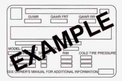
The Certification/Tire label is found on the rear edge of the driver's door. The label shows the size of your original tires and the inflation pressures needed to obtain the gross weight capacity of your vehicle. This is called Gross Vehicle Weight Rating (GVWR). The GVWR includes the weight of the vehicle, all occupants, fuel and cargo.
