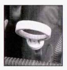
The engine oil dipstick has a yellow handle and is located near the center of the engine compartment. See Engine Compartment Overview on page 5-12 for more information on location.
