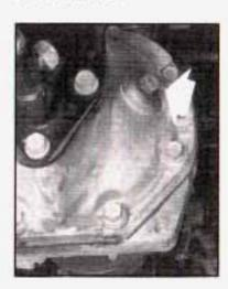
If the level is below the bottom of the filler plug hole, you may need to add some lubricant. When the differential is cold, add enough lubricant to raise the level to 3/8 inch (10 mm) below the filler plug hole.
