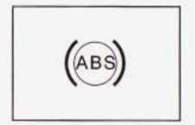
With the anti-lock brake system, this light will come on when you start your engine and may stay on for several seconds. That's normal.
