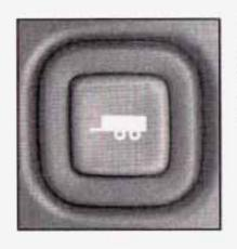
Your vehicle is equipped with a button on the instrument panel, to the right of the steering wheel, which when pressed enables tow/haul.
