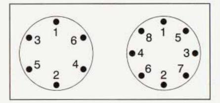
Tighten the nuts firmly in a crisscross sequence as shown. Turn the wheel wrench clockwise.
