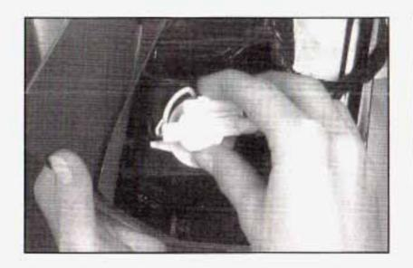
To remove, squeeze the tab on the side of the sockets while turning them counterclockwise.
