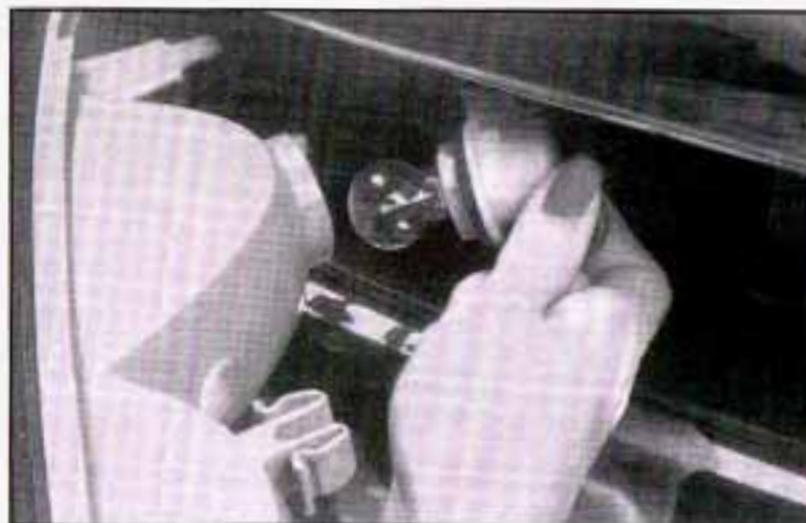
4. Turn the harness bulb socket counterclockwise to remove it. Pull the bulb straight out to remove it from the socket.
