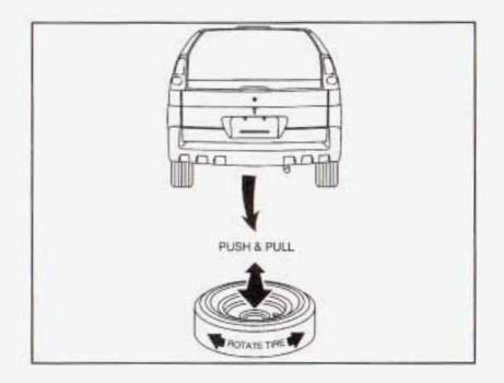
Make sure the tire is stored securely. Push, pull, and then try to rotate or turn the tire. If the tire moves, use the folding wrench to tighten the cable.
