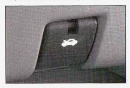
Pull the hood release handle, located on the driver's side under the instrument panel.
