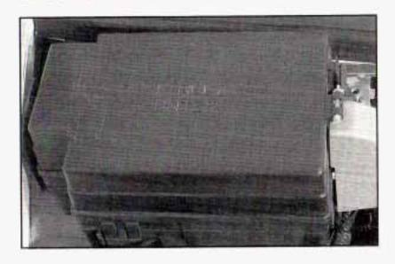
This fuse block is located in the engine compartment, on top of the windshield washer fluid reservoir.
