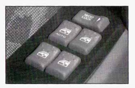
Switches on the drivers door armrest control each of the windows when the ignition is in ON, ACCESSORY, or when Retained Accessory Power is active. See "Retained Accessory Power (RAP)" under Ignition Positions on page 2-22 for more information. In addition, each passenger's door has a window switch.
