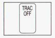
To turn the system off, press the TRAC OFF button on the instrument panel switchbank.
