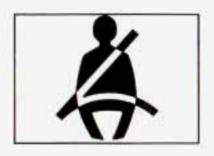
The safety belt light will also come on and stay on for several seconds. If the driver's belt is already buckled, neither the chime nor the light will come on.
