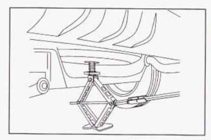
Lower the jack by turning the folding wrench counterclockwise. Keep lowering the jack until the spare tire is resting on the folding wrench.
