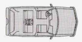
The center rear seating position has a lap-shoulder belt. To secure a child restraint in this position, you'll use only the lap part of the belt. Disconnect the shoulder part of the belt and store it before securing child restraint. See Center Rear Passenger Position on page 1-31.
