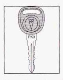
This key can be used for the ignition as well as all door locks, the liftgate/tailgate lock and the storage compartments.
