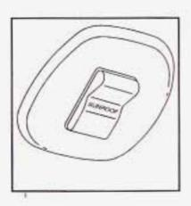
If your vehicle has a sunroof, the switch is located between the sun visors.
