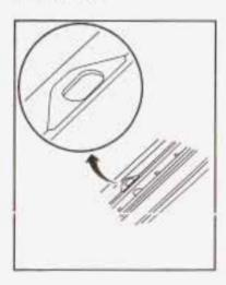
Use the four tie-down loops in each of the side rails to help secure large loads. When you are done using the crossrails you must replace the sunroof stop.
