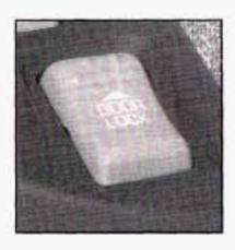
The power door lock switch is located on the driver's and front passenger's door armrest.
