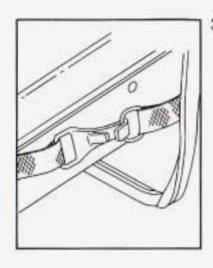
Disconnect the tethered ring from the hook and place the tethered ring on the outer edge of the tailgate on each side of the vehicle.
