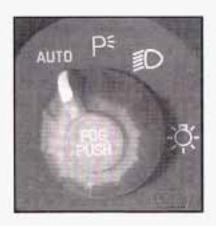
The control located to the left of the steering column operates the exterior lamps. The exterior lamp control has three positions:
