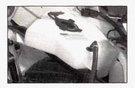
The coolant level should be at or above the FULL COLD mark. If it isn't, you may have a leak at the pressure cap or in the radiator hoses, heater hoses, radiator, water pump or somewhere else in the cooling system.
