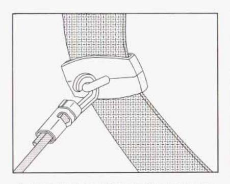
Attach the elastic cord to the comfort guide on the center passenger shoulder belt.
