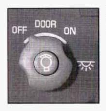
Your interior lamp control is located below the exterior lamp control.
