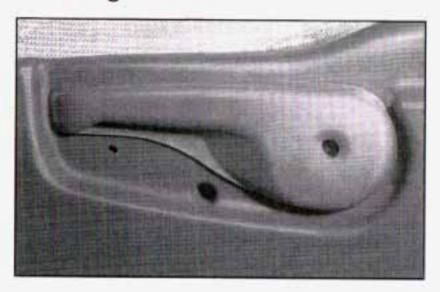
To adjust the seatback, pull up on the recliner lever located on the outboard sides of both the driver's and front passenger's seats.
