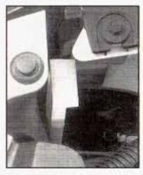
Push in on the headlamp and lift up the headlamp retaining clip partway, but do not remove.
