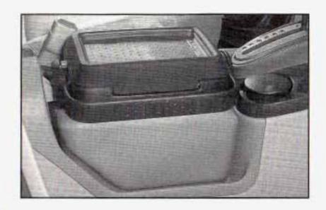
Your vehicle may have a fully insulated food/beverage console/cooler located between the driver's and front passenger's seats.
