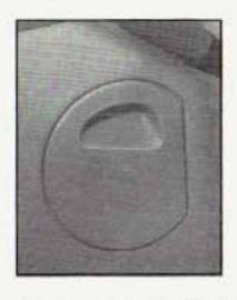
The floor console fuse block is located to the right of the shift lever.
