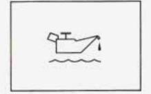
If the low engine oil level message appears on the instrument cluster, it means you need to check your engine oil level right away. For more information, see Low Engine Oil Level Message on page 3-43.
