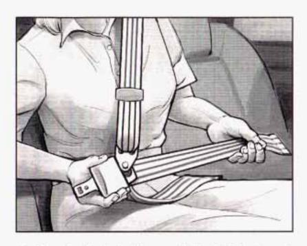
To make the lap belt longer, tilt the latch plate and pull it along the belt.
