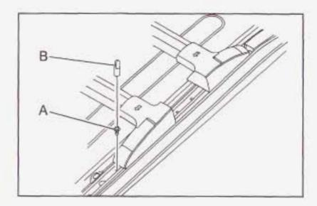
To adjust the crossrail(s), the sunroof stop (A) must be removed.
