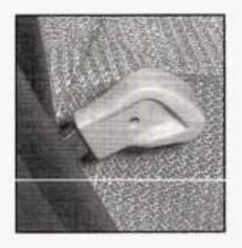
To recline the seatbacks lift up on the recliner lever located on the outboard side of the seatback. Move the seatback to the desired position.
