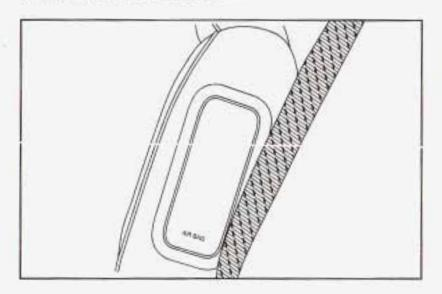
If your vehicle has a side impact air bag for the right front passenger, the words AIR BAG will appear on the air bag covering on the side of the right front passenger's seatback closest to the door.
