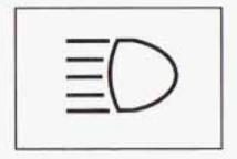
When the high beams are on, this light, on the instrument panel cluster and the HUD display, will also be on.
