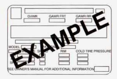
The Certification/Tire label is found on the rear edge of the driver's door. The label shows the size of your original tires and the inflation pressures needed to obtain the gross weight capacity of your vehicle. This is called the Gross Vehicle Weight Rating (GVWR). The GVWR includes the weight of the vehicle, all occupants, fuel and cargo.
