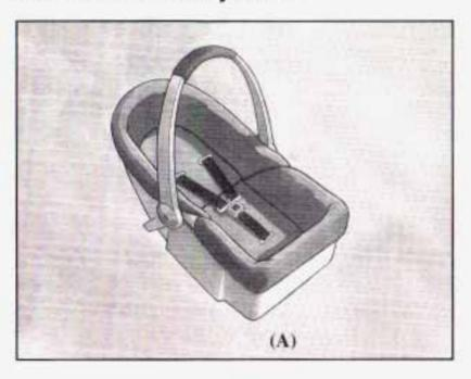
An infant car bed (A), a special bed made for use in a motor vehicle, is an infant restraint system designed to restrain or position a child on a continuous flat surface. Make sure that the infant's head rests toward the center of the vehicle.
