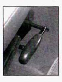
Pull up on the lever, located on the front of the seat, to unlock and move the seat.
