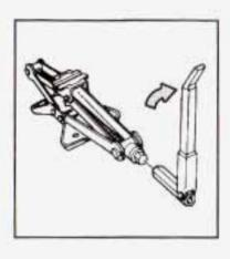
Attach the folding wrench to the jack, and turn the wrench clockwise to raise the jack head 3 inches (7.6 cm).
