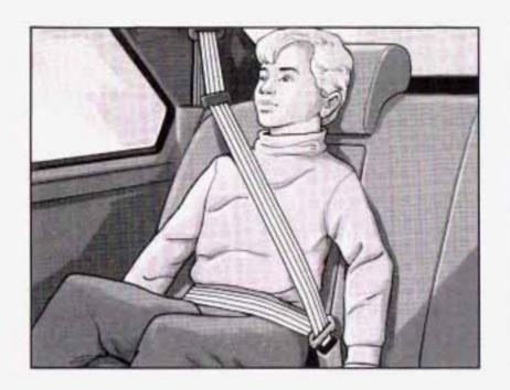
Buckle, position and release the safety belts as described in Rear Seat Passengers on page 1-28. Make sure that the shoulder belt crosses the shoulder.
