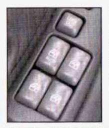
Use the switches on the driver's door armrest to operate each of the windows while the ignition is on or while Retained Accessory Power (RAP) is active. See "Retained Accessory Power (RAP)" under Ignition Positions on page 2-19 for more information.
