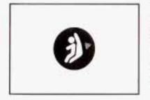
To assist you in locating the lower anchors for this child restraint system, each seating position with the LATCH system will have a dot on the seatback directly above the anchor.
