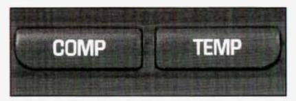
Your vehicle may have an automatic-dimming rearview mirror with a compass and temperature display.
