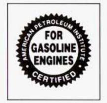
If you choose to perform the engine oil change service yourself, be sure the oil you use has the starburst symbol on the front of the oil container. If you have your oil changed for you, be sure the oil put into your engine is American Petroleum Institute certified for gasoline engines.
