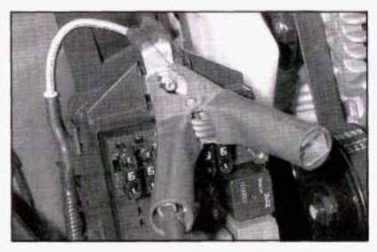
Connect the red positive (+) cable to the positive (+) terminal location on the vehicle with the dead battery. Use a remote positive (+) terminal if the vehicle has one.
