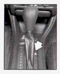
The override access slot is located on the upper right side of the console shift panel.
