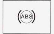
If your vehicle has the optional anti-lock brake system, this light will come on when your engine is started and may stay on for several seconds.
