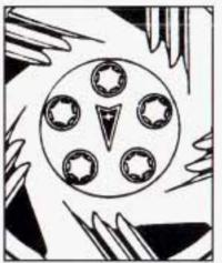
If there is a wheel cover, loosen the plastic nut caps with the wheel wrench. They won't come off. Then, using the flat end of the wheel wrench, pry along the edge of the cover until it comes off.
