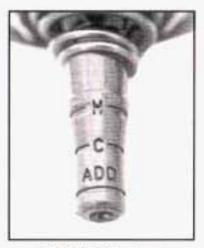
The level should be at the C (3100 V6 engine) or COLD (3800 V6 and 3800 V6 Supercharged engines) mark. If necessary, add only enough fluid to bring the level up to the mark.
