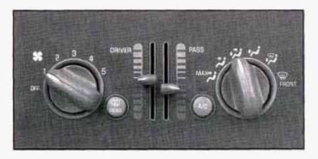
Use the mode knob located on the right side of the climate control panel to select the following modes:
