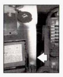
When the engine is cold, the coolant level should be at or above the COLD mark on the coolant recovery tank.
