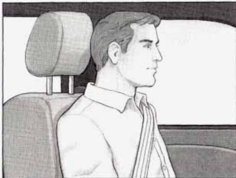
Adjust your head restraint so that the top of the restraint is closest to the top of your head. This position reduces the chances of a neck injury in a crash.
