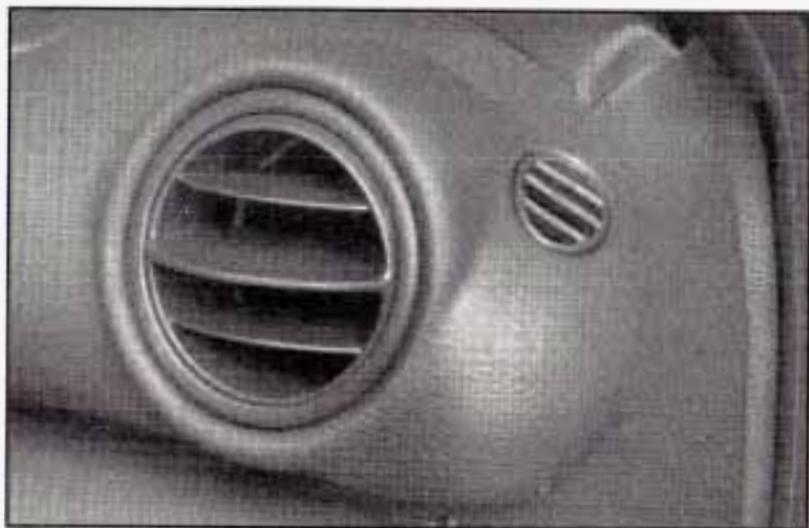
Use the louvers located on the air outlets to change the direction of the airflow.
