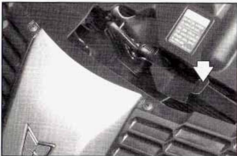
2. Then go to the front of the vehicle and lift up on the secondary hood release lever. The secondary hood release lever is located near the front center of the hood toward the driver's side.
