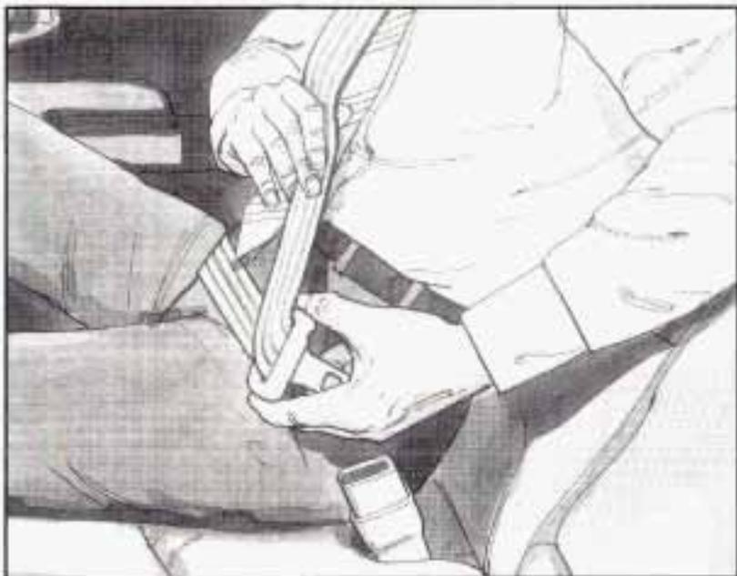
If the belt stops before it reaches the buckle, tilt the latch plate and keep pulling until you can buckle it. Pull up on the latch plate to make sure it is secure. If the belt is not long enough, see *Safety Belt Extender* on page 1-29.
