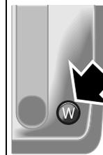
To select **Winter mode**, press the "W" button. The Winter mode facilitates starting off and driving on icy roads. Third gear is selected automatically for starting off to reduce wheelspin.
