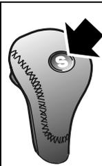
To select **Sport mode**, press the "S" button on the selector lever when the selector lever is in position N, D, 3, 2 or 1.
