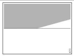
Correctly adjusted low beam
