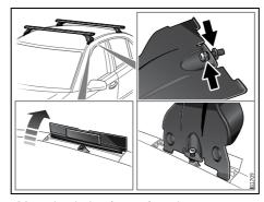
Mounting holes for roof carrier
