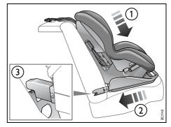
Rigid 2-point lower anchorage with top tether
