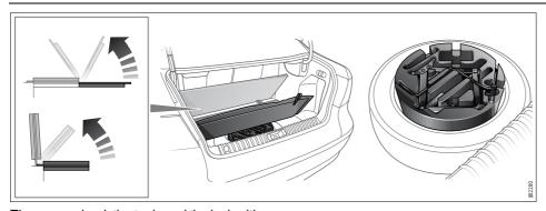
The spare wheel, the tools and the jack with its crank are carried under a panel in the trunk.
