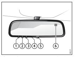
Buttons for garage opener, autodimming and compass
