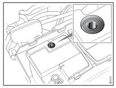
Checking the battery electrolyte level. Level correct if level indicator dark
