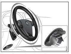
Lever for steering wheel adjustment
