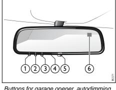
Buttons for garage opener, autodimming and compass
