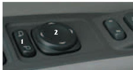
2. Press the directional arrow on the control button to move the mirror in that direction and adjust the mirror.
