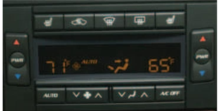
(Floor/Defog icon) appears on the display. The Floor/Defog mode directs air between the windshield, floor outlets and side windows. Press AUTO again to return to automatic operation.
