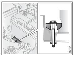
Correct position for battery clamp
