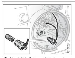
Parking-light bulb (cars with halogen low beam)
