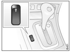
Switch for operation of central locking
