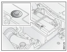
Electrolyte level indicator. Level correct if level indicator dark. Battery should be changed if indicator is light
