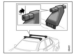
3 Start on the left-hand side of the car. Rest the carrier carefully across the roof, with the rigid foot towards you. Hold the foot clear of the roof to avoid damaging the paintwork.
