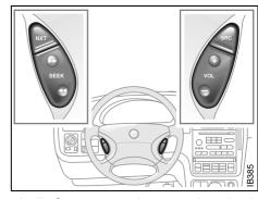
Audio System controls on steering wheel
