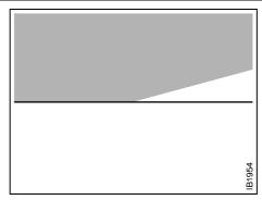
Correctly adjusted low beam
