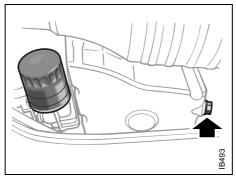
Drain plug and oil filter
