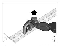
Cargo bolts mounted on the longitudinal rails
