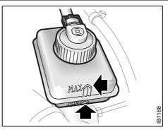
Brake and clutch-fluid reservoir
