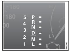
Selector-lever indicator on main instrument panel
