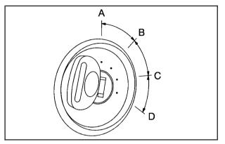
**A (OFF):** This is the only position in which you can remove the key. This position locks the ignition and transaxle.
