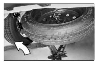
Lower the jack by turning the folding wrench counterclockwise. Keep lowering the jack until the spare tire slides off the jack.
