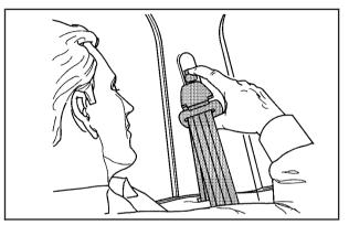
To move it down, push down on the button and move the height adjuster to the desired position.
