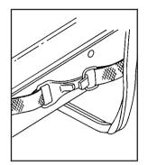
3. Disconnect the tethered ring from the hook and place the tethered ring on the outer edge of the tailgate on each side of the vehicle.
