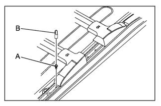
To adjust the crossrail(s), the sunroof stop (A) must be removed.
