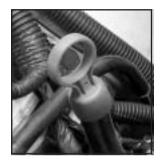
The dipstick is located toward the back of the engine compartment, next to the brake master cylinder.
