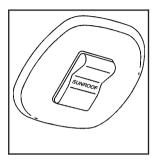
If the vehicle has a sunroof, the switch is located between the sun visors.
