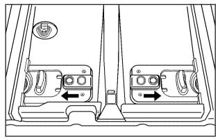
2. Insert the slide locks under the two rear floor retainers by pushing the button down and pressing them outward.
