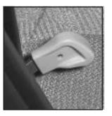
To recline the seatbacks lift up on the recliner lever located on the outboard side of the seatback.
