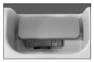
Once the liftgate is opened, reach inside the tailgate to lift the handle. Open the tailgate.
