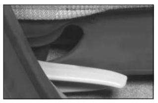
4. Pull the lever, located at the base on the outboard side of the seat, to release the rear latches from the floor pins and flip the seat forward.
