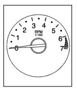
The tachometer located on your instrument panel displays the engine speed in revolutions per minute (rpm).
