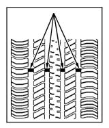
One way to tell when it's time for new tires is to check the treadwear indicators, which will appear when your tires have only 1/16 inch (1.6 mm) or less of tread remaining. You need a new tire if any of the following statements are true:
