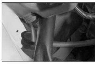
Fill the radiator with the proper DEX-COOL<sup>®</sup> coolant mixture, up to the base of the filler neck. See *Engine Coolant on page 5-23* for more information about the proper coolant mixture.
