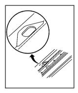
Use the four tie-down loops in each of the side rails to help secure large loads.
