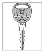
Your vehicle is equipped with the PASS-Key<sup>®</sup> III (Personalized Automotive Security System) theft-deterrent system. PASS-Key<sup>®</sup> III is a passive theft deterrent system. This means you don't have to do anything different to arm or disarm the system. It works when you insert or remove the key from the ignition.
