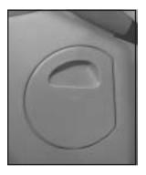
Pull the door open to access the fuse block.
