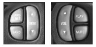
If your vehicle has this feature, some audio controls can be adjusted at the steering wheel. They include the following:
