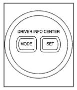
The DIC controls are located to the right of the instrument panel cluster.
