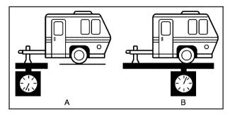
If you are using a weight-carrying or a weight-distributing hitch, the trailer tongue weight (A) should be 10 percent to 15 percent of the total loaded trailer weight (B). Do not exceed the maximum allowable tongue weight for your vehicle.
