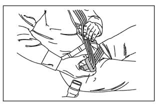
If the belt stops before it reaches the buckle, tilt the latch plate and keep pulling until you can buckle it.
