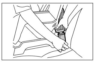
3. Buckle the belt. Make sure the release button is positioned so you would be able to unbuckle the safety belt quickly if you ever had to.
