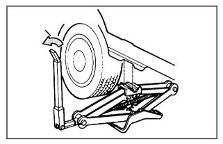
Lower the vehicle by attaching the folding wrench to the jack and turning the wrench counterclockwise. Lower the jack completely.
