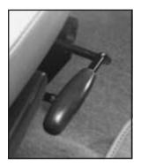
Slide the seat to where you want it and release the lever. To make sure the seat is locked into place, try to move the seat back and forth with your body.
