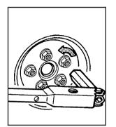
Loosen the wheel nuts — but do not remove them — using the folding wrench. Turn the handle about 180 degrees, then flip the handle back to the starting position. This avoids taking the wrench off the lug nut for each turn.
