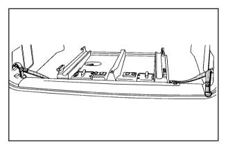
3. Feed the tethered ring upward through the lower sidewall loop on each side of the vehicle.
