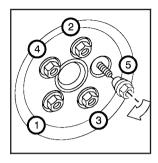
12. Tighten the wheel nuts firmly in a crisscross sequence, as shown.
