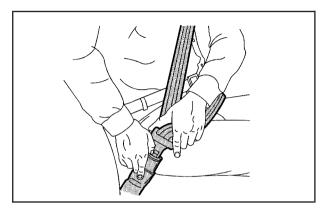
To unlatch the belt, just push the button on the buckle. The belt should go back out of the way.
