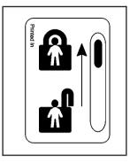
2. On the inside of the rear door will be a lock. Push the lever up to engage the safety lock.
