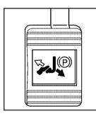
The parking brake is located under the instrument panel on the driver's side of the vehicle.
