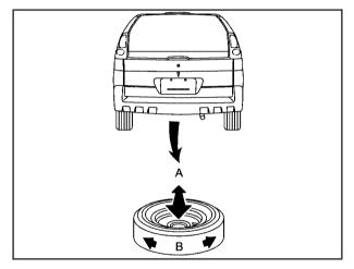
8. Make sure the tire is stored securely. Push, pull (A), and then try to turn (B) the tire. If the tire moves, use the folding wrench to tighten the cable.
