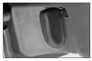
The lever that allows you to tilt the steering wheel is located on the left side of the steering column. To tilt the wheel, hold the wheel and pull the lever. Then move the wheel to a comfortable position and release the lever to lock the wheel in place.
