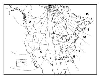
**ZONE - PRESS & HOLD SET TO CHANGE:** This display mode will appear when you are manually calibrating the system. When the compass is being recalibrated for the first time, the zone symbol will be displayed. When the compass is being recalibrated any time after that, the current zone number for compass variance will be displayed in place of the zone symbol. Use the SET button to select the zone number from the graphic shown to select the current area of the country that you are driving in.
