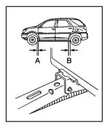
Locate the notch (A is 3.0 inches (7.5 cm) from the front tire or B is 5.5 inches (14.0 cm) from the rear tire) in the frame. The notch is located near each wheel in the vehicle's body.
