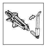
Attach the folding wrench to the jack, and turn the wrench clockwise to raise the jack head 3 inches (7.6 cm).
