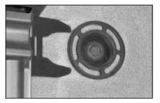
1. Slide the floor track assembly in while aligning the front forks, located on the bottom front of the track assembly, so that the forks slide under the two front floor retainers.
