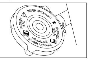
You can remove the radiator pressure cap when the cooling system, including the radiator pressure cap and upper radiator hose, is no longer hot. Turn the pressure cap slowly counterclockwise until it first stops. Do not press down while turning the pressure cap.
