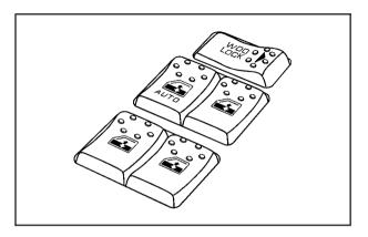
Switches on the driver's door armrest control each of the windows when the ignition is in ON, ACCESSORY, or when Retained Accessory Power (RAP) is active. See *Retained Accessory Power (RAP) on page 2-20* for more information. In addition, each passenger's door has a window switch. The driver's power window switch has two down positions. Push the rear of the switch to the first position to lower the window to the desired level.
