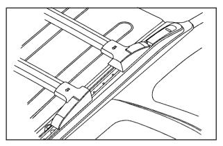
*Notice:* Loading cargo on the luggage carrier that weighs more than 220 lbs (100 kg) or hangs over the rear or sides of the vehicle may damage your vehicle. Load cargo so that it rests on the slats as far forward as possible and against the side rails, making sure to fasten it securely.
