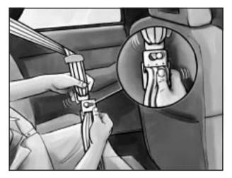
Insert the metal knob on the shoulder belt into the keyhole on the lap belt buckle as shown. Be sure to slide the shoulder belt part into the keyhole until it locks into place.
