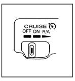
The cruise controls are located on the end of the turn signal/multifunction lever.
