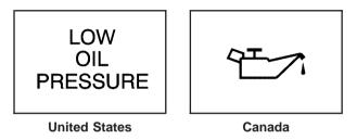
Your vehicle is equipped with a low oil pressure warning message.
