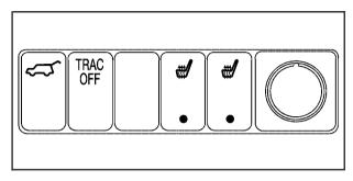
There is an instrument panel switchbank located below the comfort controls. It contains switches or blanks that will vary with the options that are on your vehicle and a cigarette lighter/accessory power outlet.
