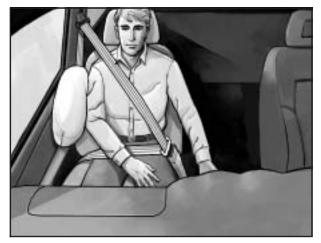
If your vehicle has one, the right front passenger's side impact airbag is in the side of the passenger's seatback closest to the door.
