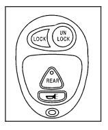
With this feature, you can lock and unlock your doors using the remote keyless entry transmitter supplied with your vehicle.
