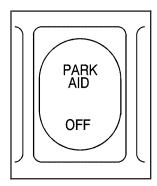
URPA can be turned off by pressing the rear park aid disable switch located in the instrument panel switchbank. When the system is disabled, an indicator light will glow on the switch. You will not see any lights on the rear display if the switch is in the off position.
