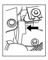
Push in on the headlamp panel and lift up the headlamp retaining clip partway, but do not remove.
