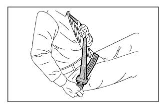
To make the lap part tight, pull down on the buckle end of the belt as you pull up on the shoulder part.
