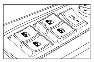
Switches on the driver's door armrest control each of the windows when the ignition is in ON, ACCESSORY, or when Retained Accessory Power (RAP) is active. See *Retained Accessory Power (RAP) on page 2-20* for more information. In addition, each passenger's door has a window switch.
