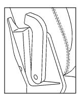
For up-level split bench seats, continue pushing forward on the recliner lever to release the rear latches from the floor pins and flip the seat forward.
