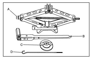
The tools you will be using include the jack (A), folding wrench (B), wing nut (C), and J-hook (D).
