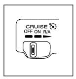
The cruise controls are located on the end of the turn signal/multifunction lever.
