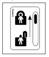
On the inside of the rear door will be a lock. Push the lever up to engage the safety lock.
