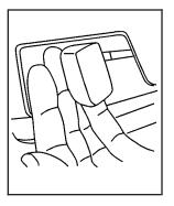
To tilt the wheel, hold the wheel and pull the lever. Then move the wheel to a comfortable position and release the lever to lock the wheel in place.
