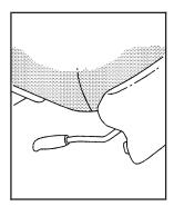
Use the lever located under the front of the seat to adjust the seat forward or rearward.
