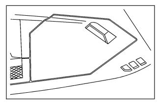
The floor console fuse block is located to the left of the glove box near the floor. Pull the door open to access the fuse block.
