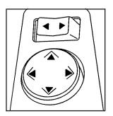
The power mirror controls are located on the driver's door armrest.
