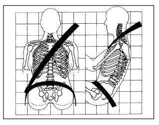
The lap part of the belt should be worn low and snug on the hips, just touching the thighs. In a crash, this applies force to the strong pelvic bones. And you would be less likely to slide under the lap belt. If you slid under it, the belt would apply force at your abdomen. This could cause serious or even fatal injuries. The shoulder belt should go over the shoulder and across the chest. These parts of the body are best able to take belt restraining forces.
