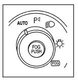
The control on the left side of the steering column operates the exterior lamps.
