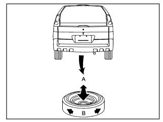
Make sure the tire is stored securely. Push, pull (A), and then try to turn (B) the tire. If the tire moves, use the folding wrench to tighten the cable.  Put back all tools as they were stored in the jack storage compartment and put the compartment cover back on.
