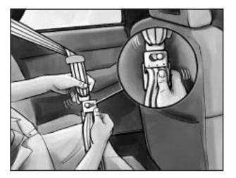
Insert the metal knob on the shoulder belt into the keyhole on the lap belt buckle as shown. Be sure to slide the shoulder belt part into the keyhole until it locks into place.
