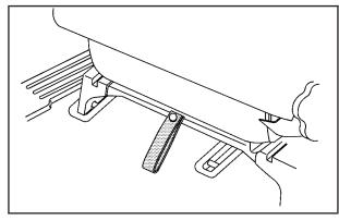
3. Pull the nylon strap behind the chair to release the rear hooks from the floor pins.
