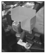
If your vehicle has the 3.6L V6 engine, pull up on the cap to access the remote positive (+) terminal.
