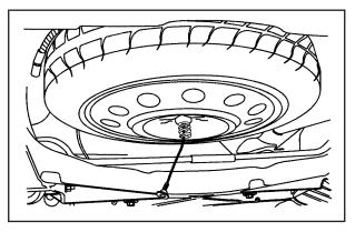
If the spare tire will not lower, the secondary latch may be engaged causing the tire not to lower.
