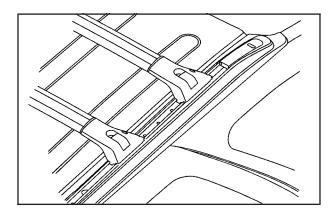
Notice: Loading cargo on the luggage carrier that weighs more than 220 lbs (100 kg) or hangs over the rear or sides of the vehicle may damage your vehicle. Load cargo so that it rests on the slats as far forward as possible and against the side rails, making sure to fasten it securely.
