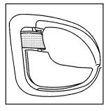
To unlock either manual locking front door from the inside, pull back on the manual lever. To lock either front door from the inside, push the manual lever forward.
