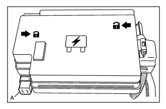
This fuse block is located in the engine compartment, on the passenger's side of the vehicle. See *Engine Compartment Overview on page 5-10* for more information on location.
