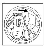
Turn the bulb socket one-quarter of a turn clockwise.
