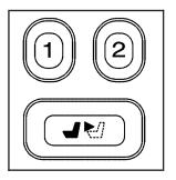
If your vehicle has this feature, the controls are located on the driver's door panel and are used to store and recall the driver's seat position and the outside rearview mirror position.
