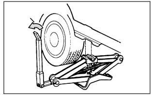
Lower the vehicle by attaching the folding wrench to the jack and turning the wrench counterclockwise. Lower the jack completely.
