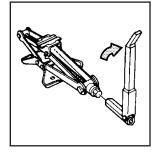
Attach the folding wrench to the jack, and turn the wrench clockwise to raise the jack head 3 inches (7.6 cm).
