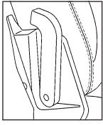
To recline the seatback on up-level split bench seats, push forward on the recliner lever located on the outboard side of the seatback.
