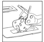
bench seat is angled so that the front hooks clear the floor pins. If the front legs are not attached correctly, the rear legs will not attach to the rear set of floor pins.
