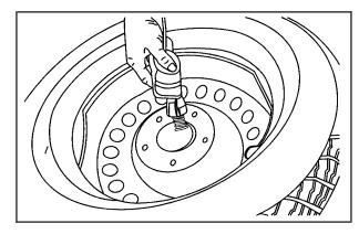
Tilt the retainer and slip it through the wheel opening to remove the spare tire from the cable. 5. Turn the wrench clockwise to raise the cable back up after removing the spare tire.
