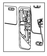
The equipment you will need is located in the storage compartment on the passenger's side, at the rear of the vehicle.
