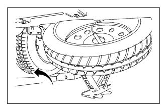
Lower the jack by turning the folding wrench counterclockwise. Keep lowering the jack until the spare tire slides off the jack.
