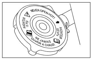
You can remove the radiator pressure cap when the cooling system, including the radiator pressure cap and upper radiator hose, is no longer hot. Turn the pressure cap slowly counterclockwise until it first stops. Do not press down while turning the pressure cap.
