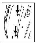
2. Remove the two screws on the inboard taillamp panel.
