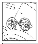
While refueling, hang the tethered fuel cap from the hook on the fuel door.
