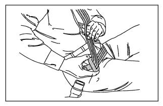
If the belt stops before it reaches the buckle, tilt the latch plate and keep pulling until you can buckle it.
