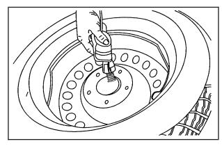
5. Tilt the retainer and slip it through the wheel opening to remove the spare tire from the cable.
