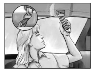
Remove the shoulder belt from its stowage location in the roof and pull it all the way down to the lap belt.
