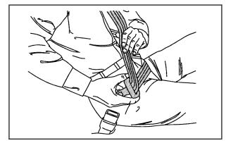
If the belt stops before it reaches the buckle, tilt the latch plate and keep pulling until you can buckle it. Pull up on the latch plate to make sure it is secure.
