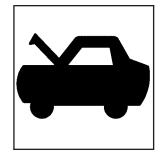
Pull the hood release handle with this symbol on it. It is located under the instrument panel on the driver's side of the vehicle.
