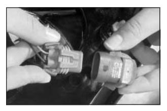
Unhook the electrical connector by lifting up the gray tabs and separate the connector from the bulb base.
