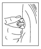
3. Remove the seven wing nuts and the four outboard nuts (two at each end).
