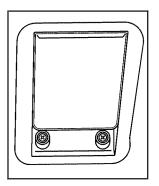
To fold the seatback down, pull up on the lever located on the back of the seat. Push down on the seatback until it is locked into place.
