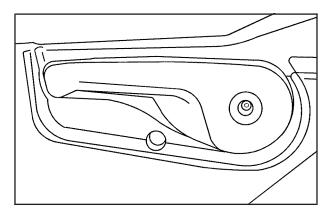
To recline the seatback, lift up on the recliner lever located on the outboard side of the seatback. Use the recliner lever to move the seatback to the desired position.
