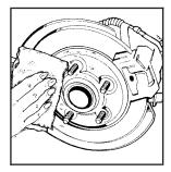
Remove any rust or dirt from the wheel bolts, mounting surfaces and spare wheel. 10. Place the compact spare tire on the wheel-mounting surface.
