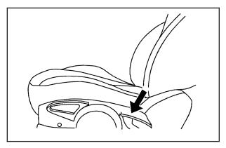
Your vehicle has reclining seatbacks. The lever is located on the outboard side of the seats. Lift the lever to release the seatback. Move the seatback to where you want it and release the lever to lock the seatback in place. Press rearward on the seatback to be sure it is locked into place.
