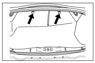
Open the trunk and pull one or both of the small handles located in the center of the trunk.
