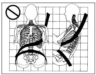
A: The shoulder belt is worn under the arm.
