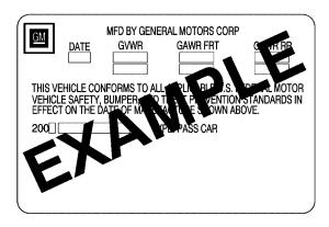
A vehicle specific Certification label, found on the rear edge of the driver's door, tells you the gross weight capacity of your vehicle, called the Gross Vehicle Weight Rating (GVWR). The GVWR includes the weight of the vehicle, all occupants, fuel, and cargo. Never exceed the GVWR for your vehicle, or the Gross Axle Weight Rating (GAWR) for either the front or rear axle.
