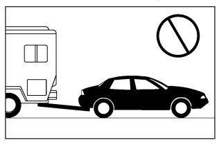
Notice: Towing your vehicle from the rear could damage it. Also, repairs would not be covered by the warranty. Never have your vehicle towed from the rear.
