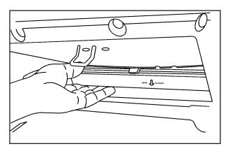
4. Remove the filter by sliding it out of the housing.
