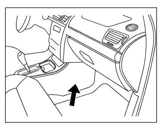
The floor console fuse block is located on the passenger's side of the floor console under the instrument panel. To access the fuse block, remove the panel on the side of the console.
