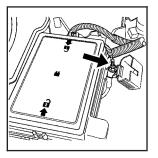
The remote positive (+) terminal is located under a red plastic cover on the engine compartment fuse block. Open the cover to access the terminal.
