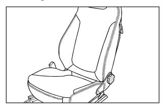
To adjust the seatback, turn the knob on the outboard side of the seatback until the seatback is in the desired position.
