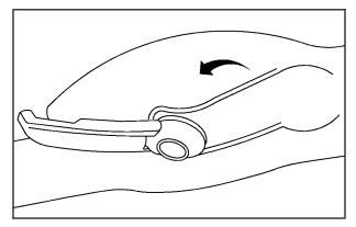
The convertible top front latch, located above the inside rearview mirror, must be unlatched. Pull the latch down and turn it counterclockwise to unlatch it. Leave the latch open and rotated to prevent damage.
