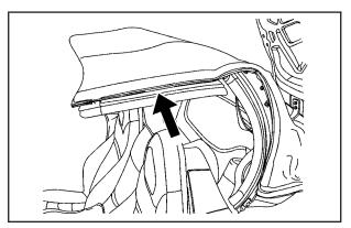
Pull the convertible top forward by firmly gripping the side edge (B) and applying a brisk upward and forward motion to get the top in the pull-up position. Close the trunk (D) by pushing it down with a swift, firm motion.
