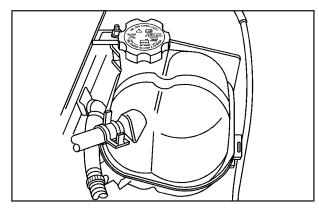
The coolant surge tank is located in the engine compartment on the driver's side of the vehicle. See *Engine Compartment Overview on page 5-12* for more information on location.
