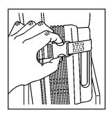
Remove the tire inflator kit strap by squeezing the two tabs of the quick release buckle.
