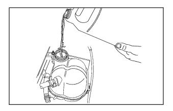
3. Fill the coolant surge tank with the proper mixture, to the COLD FILL line. Wait about five minutes, then check to see if the level is below the COLD FILL line. If the level is below the line, add additional coolant to bring the level up to the line. Repeat this procedure until the level remains constant at the COLD FILL line for at least five minutes.
