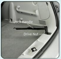
Lift up the cover and fit the jack-handle over the drive nut. Rotate the nut to the left until you can remove the swivel hook from the stowage basket. Swing the basket down to remove the compact spare tire.
