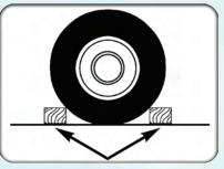
Block both the front and rear of the wheel diagonally opposite the jacking position.
