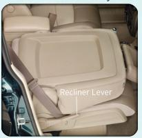
The front passenger seat can be folded flat. Pull up on the recliner lever, to the full upward position, to fold down the seat back.
