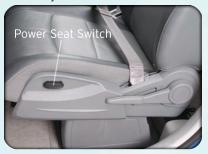
The power seat switch is located on the outboard side of the seat near the floor.
