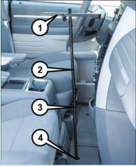
• Using the provided tools, lower the spare tire by turning the "spare tire drive" nut, located on the floor in front of the floor console, counter-clockwise.
