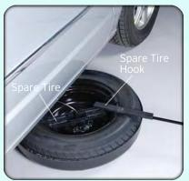
• Retrieve the spare tire from under the vehicle with the provided spare tire hook.
