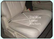
• Loosen the adjusters on the lower child restraint attachment straps to ease the installation.
