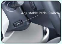
• Press the switch located on the left side of the steering column forward to move the brake and accelerator pedals away from the driver and press the switch rearward to move the pedals closer to the driver.
