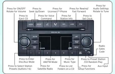
**NOTE:** Uconnect<sup>™</sup> Phone and Voice Command are vehicle options which must be ordered separately. The buttons on the radio will only be active if the vehicle has been equipped with the option.
