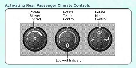
• Rotate the rear blower control, located on the main climate control in the instrument panel, to the "RR" position. This enables the rear passenger climate controls located in the headliner above the second row seats.
