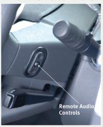
The remote audio controls are located on the rear surface of the steering wheel.
