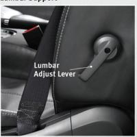
The lumbar adjust lever is on the outboard side of the seatback. Rotate the lumbar adjust lever downward to increase the lumbar support or upward to decrease the lumbar support as desired.
