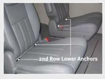
Loosen the adjusters on the lower child restraint attachment straps to ease the installation.
