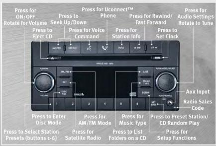
**NOTE:** Uconnect<sup>™</sup> Phone and Voice Command are vehicle options which must be ordered separately. The buttons on the radio will only be active if the vehicle has been equipped with the option.
