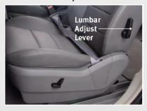
Rotate the lumbar adjust lever downward to increase the support or upward to decrease the support.
