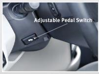
Press the switch located on the left side of the steering column forward to move the brake and accelerator pedals away from the driver and press the switch rearward to move the pedals closer to the driver.
