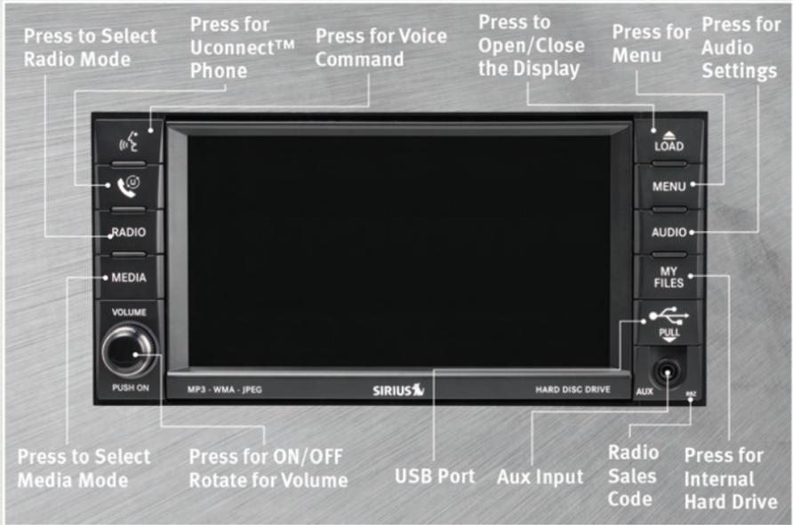
**NOTE:** Uconnect™ Phone and Voice Command are vehicle options which must be ordered separately. The buttons on the radio will only be active if the vehicle has been equipped with the option.
