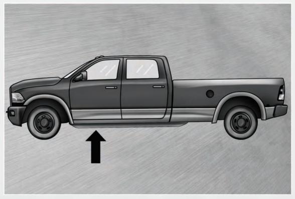
• For **4x4 front wheels,** place the jack under the axle as close to the tire as possible with the drive tubes extending to the front.
