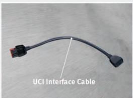
This feature allows you to plug an iPod<sup>®</sup> into the vehicle's sound system through a 16-pin connector using the provided interface cable.
