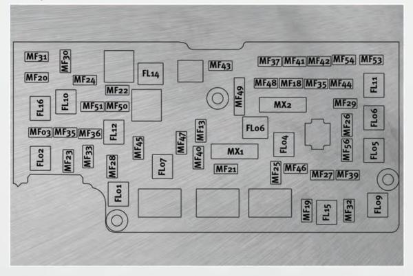
• The Totally Integrated Power Module (TIPM) is located in the engine compartment near the battery. This center contains cartridge fuses and mini fuses.
