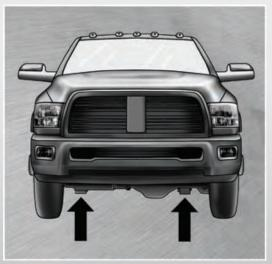
• For **rear wheels**, place the jack under the axle between the spring and the shock absorber with the drive tubes extending to the rear.
