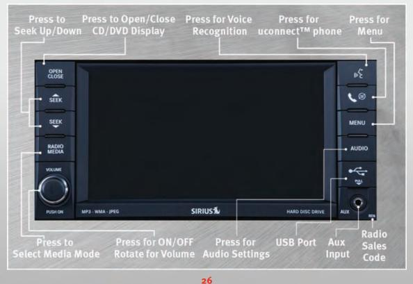
**NOTE:** uconnect<sup>™</sup> phone and Voice Recognition are vehicle options which must be ordered separately. The buttons on the radio will only be active if the vehicle has been equipped with the option.
