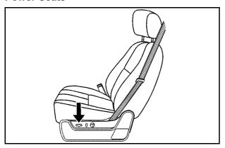
The power seat controls are located on the outboard side of the front seats.
