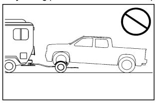
Notice: If a two-wheel-drive vehicle is towed with the rear wheels on the ground, the transmission could be damaged. The repairs would not be covered by the vehicle warranty. Never tow the vehicle with the rear wheels on the ground. Two-wheel-drive vehicles should not be towed with the rear wheels on the ground. Two-wheel-drive transmissions have no provisions for internal lubrication while being towed.
