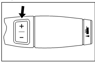
On vehicles with a Range Selection Mode, this feature may be used to control the vehicle's transmission.
