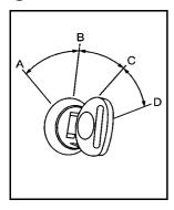
The ignition switch has four different positions.
