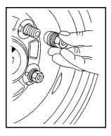
7. Put the wheel nuts back on with the rounded end of the nuts toward the wheel after mounting the spare. Tighten each wheel nut by hand. Then use the wheel wrench to tighten the nuts until the wheel is held against the hub.
