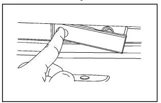
Access the storage area by pressing and holding in the driver side of the handle and pull out on the exposed portion of the handle.
