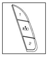
The controls for this feature are located on the driver's door, and are used to program and recall memory settings for the driver's seat, outside mirrors, steering wheel position, and the adjustable throttle and brake pedal feature, if your vehicle has it.
