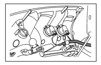
Press the release tab, if the vehicle has one, and turn the bulb socket counterclockwise to remove it from the taillamp housing.
