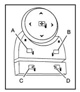
Vehicles with outside power foldaway mirrors have controls located on the driver door.
