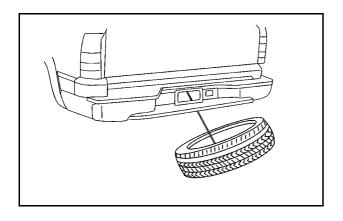
Tilt the tire toward the vehicle with some slack in the cable to allow access to the tire/wheel retainer (D). Separate the retainer from the guide pin by sliding the retainer up the pin while pressing down on the latch.
