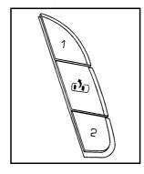
The controls for this feature are located on the driver door, and are used to program and recall memory settings for the driver seat, outside mirrors, steering wheel position, and the adjustable throttle and brake pedal feature, if the vehicle has it.
