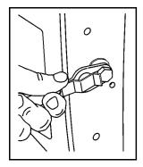
Raise the tailgate slightly and release both retaining cable clips. To release the retaining cable clips, lift the cable so it points straight out. Lift the clip over the bolt, and push the cable forward then rotate down.
