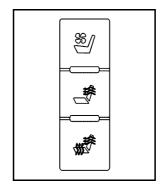
If the front seats have the heated and cooled seat feature, the buttons used to control this feature are located on the climate control panel.
