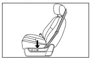
To increase lumbar support, press and hold the front of the control. To decrease, press and hold the rear of the control.
