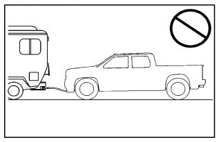
Notice: If a two-wheel-drive vehicle is towed with all four wheels on the ground, the transmission could be damaged. The repairs would not be covered by the vehicle warranty. Do not tow a two-wheel-drive vehicle with all four wheels on the ground.
