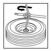
Use the wheel wrench which has a hook that lets you pull the hoist cable toward you to assist in reaching the spare tire.
