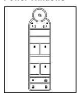
If available, the power window switches are located on each of the side doors in the front and rear, if equipped.
