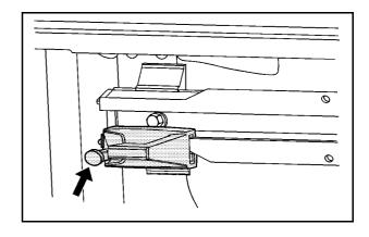
To adjust a tie-down, pull the locator pin out and move the tie-down to another location making sure the locator pin lines up with a locator hole on the rail. The tie-down pin may not be installed correctly if the pin does not line up, turn it over and reinstall. The tie-down will not move when the pin is completely installed. The maximum load for each rail is 500 lbs (227 kg).
