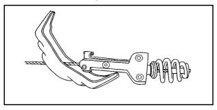
Separate the tire/wheel retainer (D) from the guide pin. Pull the pin through the center of the wheel. Tilt the retainer down and through the center wheel opening.
