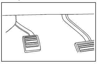
Set the parking brake by holding the regular brake pedal down, then pushing down the parking brake pedal. If the ignition is on, the brake system warning light will come on. See *Brake System Warning Light on* page 4-34.
