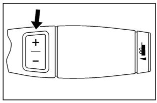
The Range Selection Mode switch is located on the shift lever. To enable the Range Selection feature, move the column shift lever to the M (Manual) position. The current range will appear next to the M. This is the highest attainable range with all lower gears accessible. As an example, when 4 (Fourth) gear is selected, 1 (First) through 4 (Fourth) gears are available.
