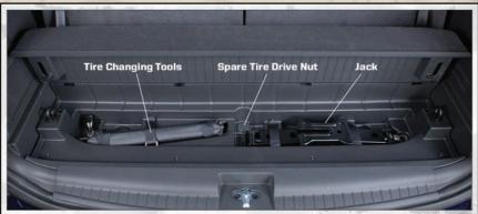
The scissor-type jack and tire changing tools are located in a compartment behind the third row seat.
