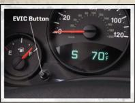
Press the EVIC button, located below the speedometer, until Personal Settings is displayed on the EVIC. Use the EVIC button to select one of the following, then press and hold the EVIC button to select either "ON" or "OFF".
