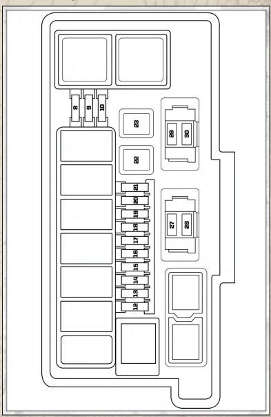
• The Integrated Power Module (IPM) is located in the engine compartment near the battery. This center contains cartridge fuses, mini-fuses and relays.
