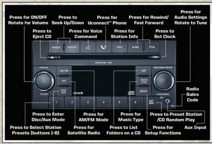
NOTE: Uconnect $^{\text{TM}}$  Phone and Voice Command are vehicle options which must be ordered separately. The buttons on the radio will only be active if the vehicle has been equipped with the option.
