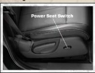
The power seat switch controls forward/back adjustment.
