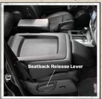
The front passenger seat can be folded flat to allow for extended cargo space. Pull up on the seatback release lever to fold down the seatback.
