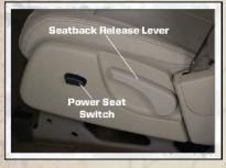
The power seat switch, located on the outboard side of the seat near the floor, controls forward/back, up/down, and tilt adjustment. Lift the seatback release lever, lean back and release at the desired position.
