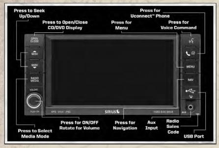
NOTE: Uconnect<sup>TM</sup> Phone and Voice Command are vehicle options which must be ordered separately. The buttons on the radio will only be active if the vehicle has been equipped with the option.
