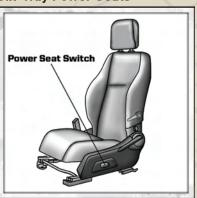
The power seat switch is located on the outboard side of the seat near the floor. Use the switch to move the seat up, down, forward, rearward, or to tilt the seat.
