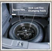
The jack and jack-handle are stowed under the load floor in the trunk.
