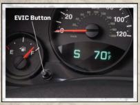
Press the EVIC button, located below the speedometer, until Personal Settings is displayed on the EVIC. Use the EVIC button to select one of the following, then press and hold the EVIC button to select either "ON" or "OFF".
