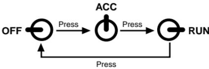
**NOTE:** If the ignition switch is left in the ACC or ON/RUN (engine not running) position and the transmission is in PARK, the system will automatically time out after 30 minutes of inactivity and the ignition will switch to the OFF position.
