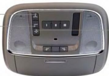
The power sunroof switches are located on the overhead console.
