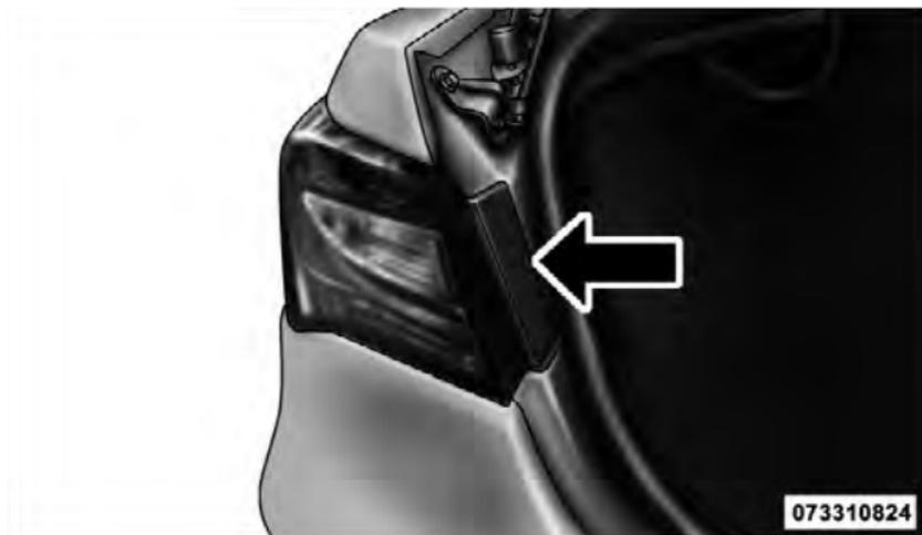
4. Twist and remove socket from lamp.
