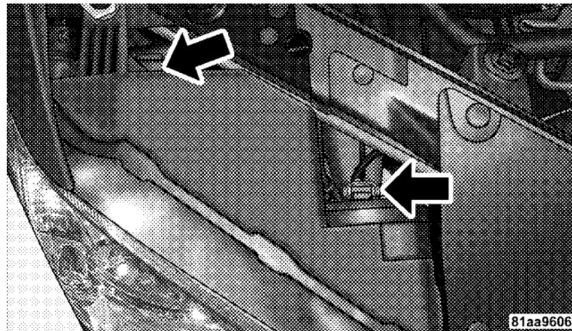
3. Rotate bulb and connector one-quarter turn and pull outward from assembly.
