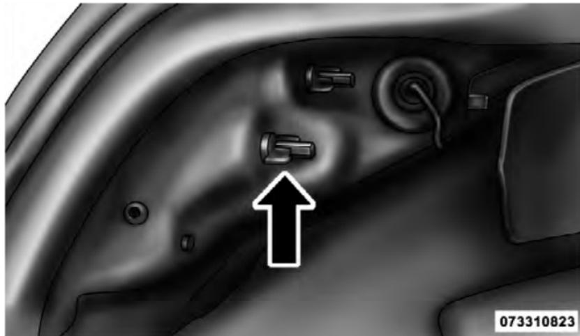
**NOTE:** Placing a small flat head screwdriver or similar tool between the lamp outboard ball stud and plastic grommet from inside the trunk can help to disengage the outboard edge of the tail lamp.
