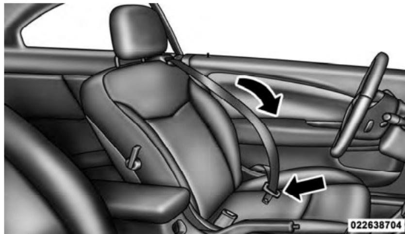
Inserting Latch Plate Into Buckle
