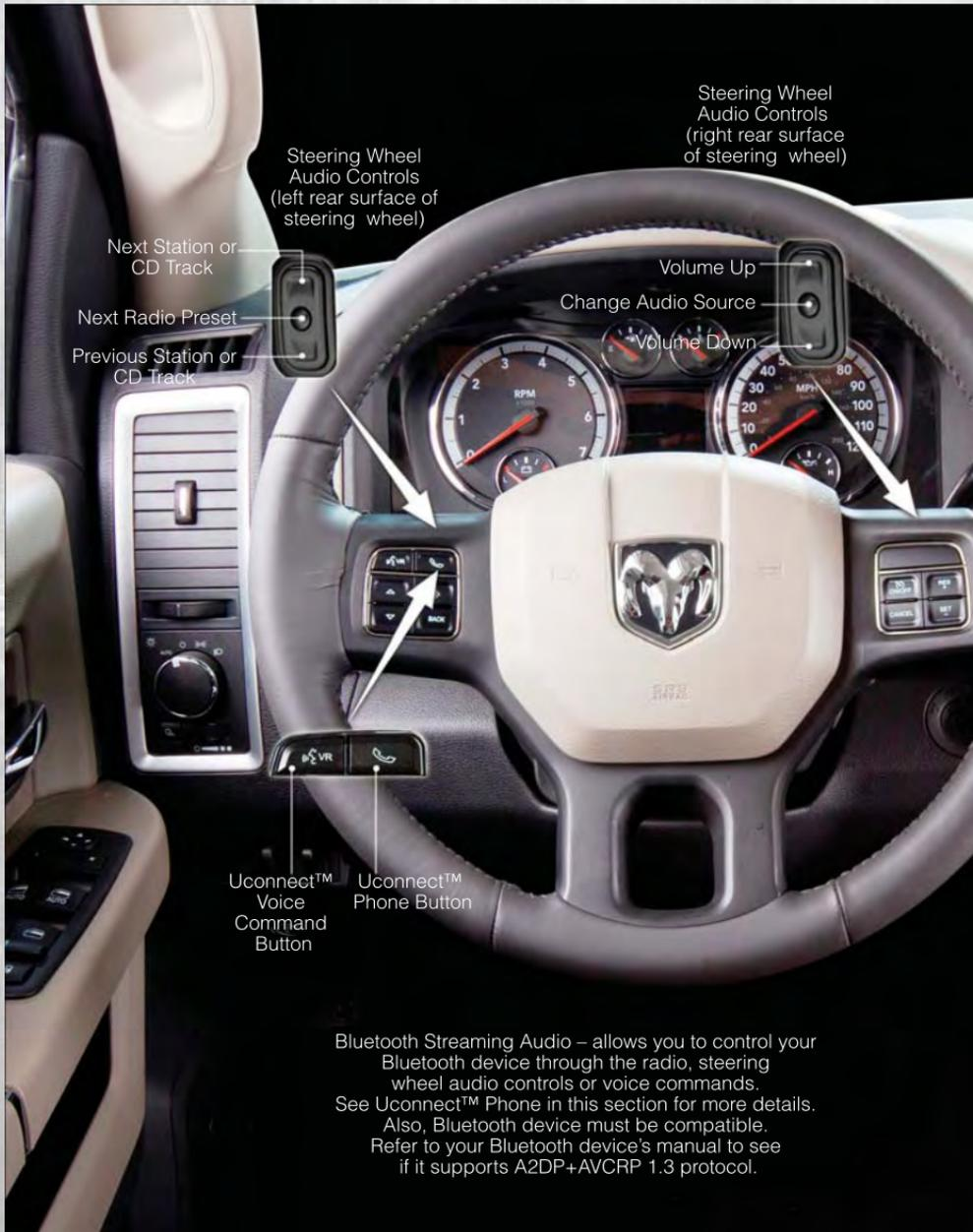
Steering Wheel Audio Controls (left rear surface of steering wheel)
