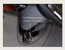
• Pull up on the handle to lock the column firmly in place.
