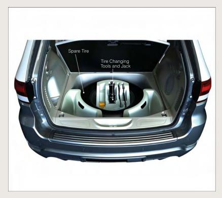
The scissor-type jack and tire changing tools are located in rear cargo area, below the load floor.
