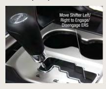
(+) will decrease or increase the top available gear. To disable ERS, simply hold the shift lever to the right (+) until "D" is again displayed in the instrument cluster.
