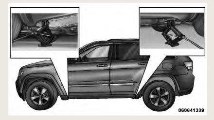
4. For the front axle, place the jack on the body flange just behind the front tire as indicated by the triangular lift point symbol on the sill molding.
