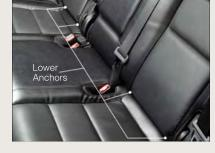
be readily identified by the symbol \( \bigcirc \) located on the seatback directly above the anchorages and are just visible when you lean into the rear seat to install the child restraint.
