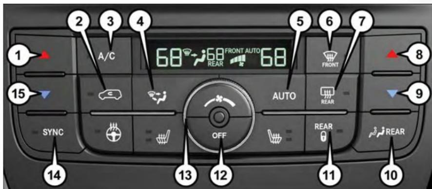
Three Zone Automatic Temperature Controls (ATC)
