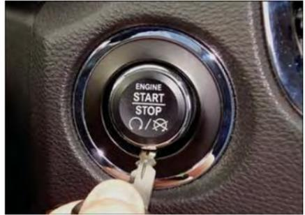
ENGINE START/STOP Button Removal
