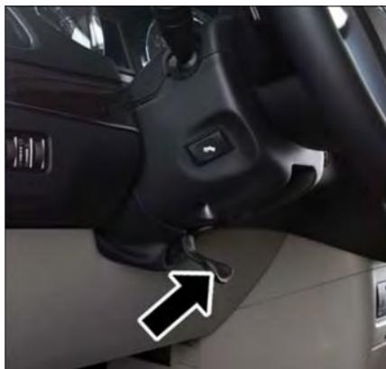
Tilt/Telescoping Steering Column Lever
