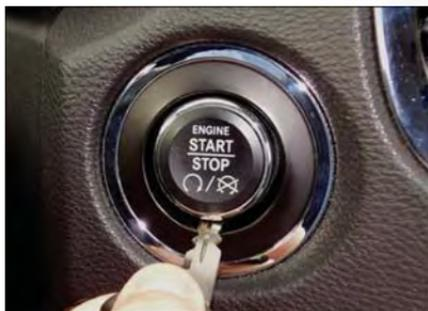
Engine START/STOP Button Removal
