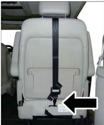
Rear Seat Tether Strap Mounting (Second Row Anchorage Shown)
