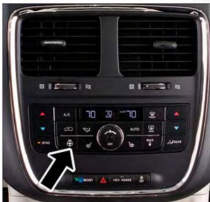
Heated Steering Wheel Switch Location
