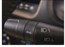
High Beam And Turn Signal Controls
