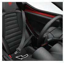
Inserting Latch Plate Into Buckle
